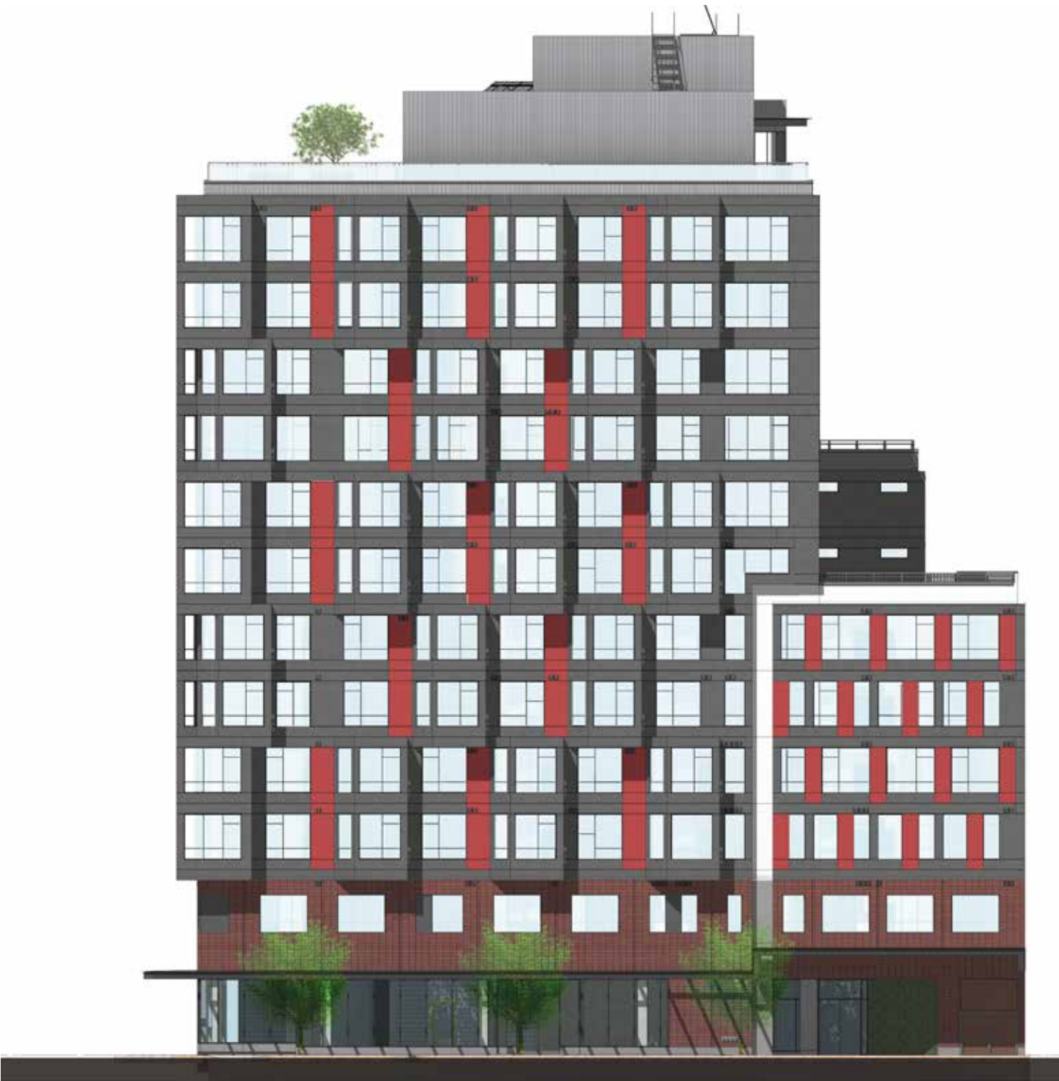
CURRENT PROPOSED ELEVATION - WINDOW WALL ON EAST AND NORTH FACADES 39.7% TOTAL GLAZED
