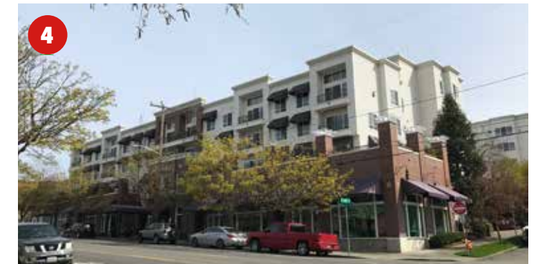
4 University House [assisted living/ mixed-use] - Retail base distinct from upper level massing
