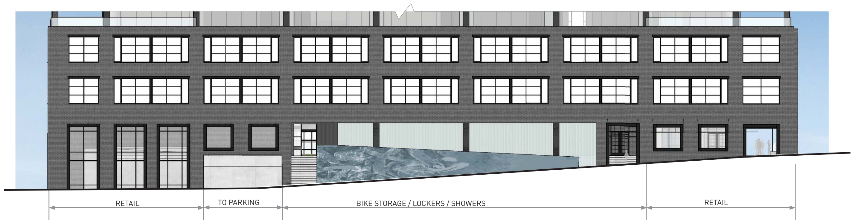
2 NORTH ELEVATION - VALLEY STREET ACCESS
