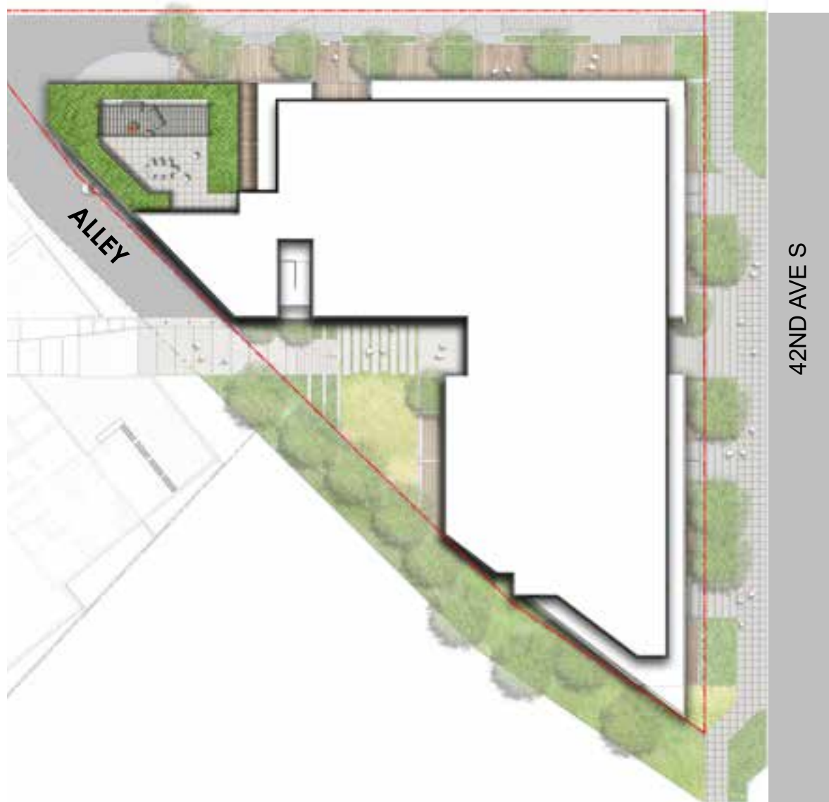
SITE B ROOF PLAN ROOF DECK CARVES AWAY NW CORNER
