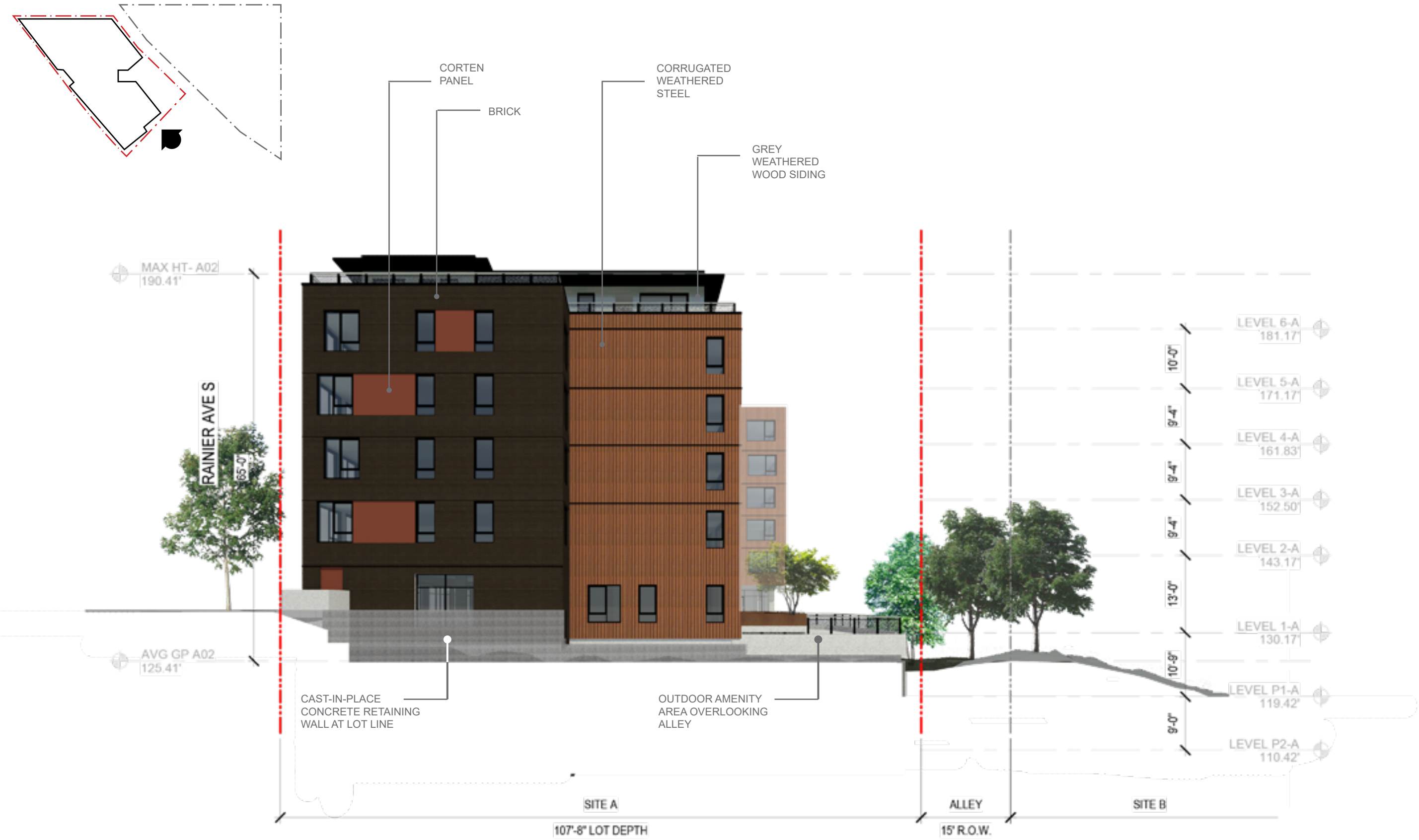
SOUTH ELEVATION ALONG SOUTH LOT LINE JUNE 21ST @ 9AM
