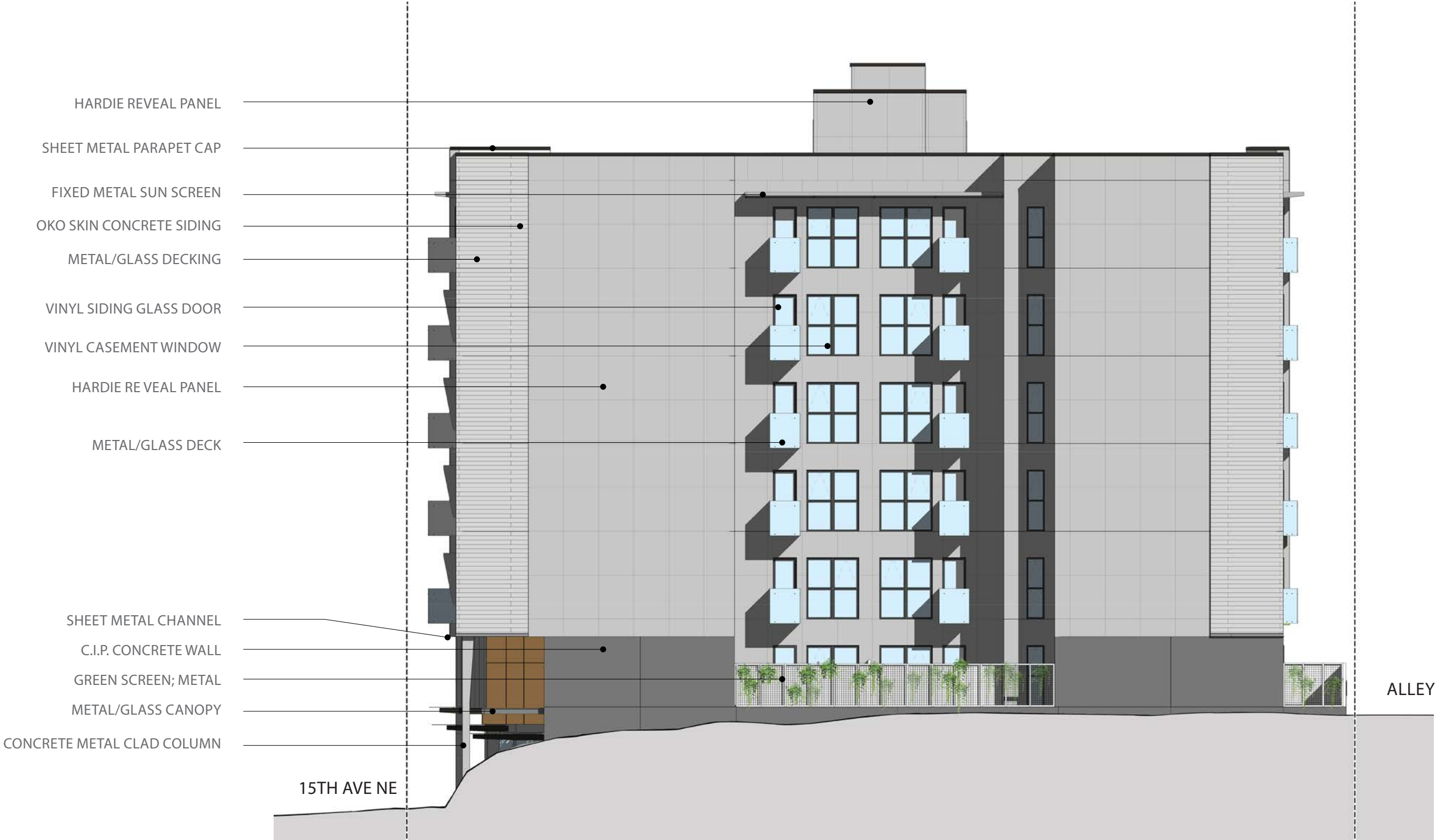
South Elevation Along Adjacent Property
