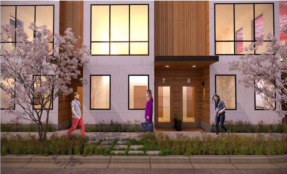
The proposed residential entries along SW 100th St and California Ave SW are close to the sidewalk grade to reduce the overall height of each building and improve unit accessibility goals for the residents.
