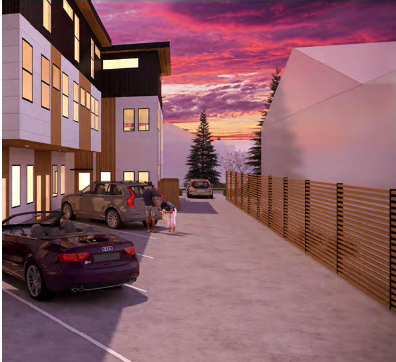
HORIZONTAL 2 X 2 CEDAR FENCE AT NORTH PROPERTY LINE SPACED AT 4" O.C. WITH VERTICAL STEEL POSTS
