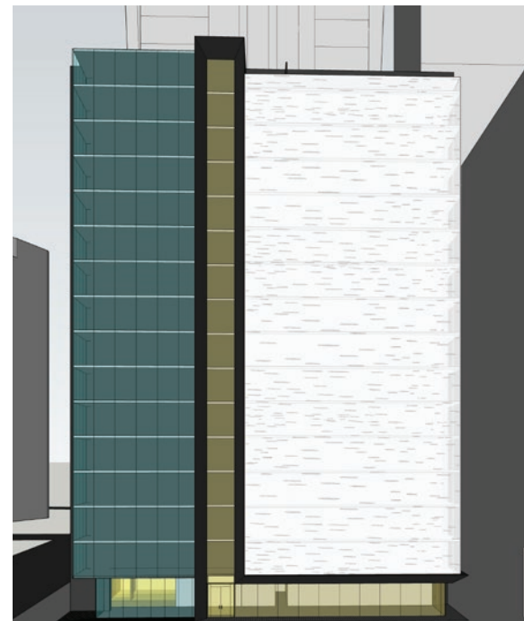
First iteration of literal birch pattern in perforated metal over curtain wall in previous design
