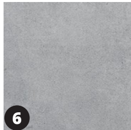
6 EXPOSED CONCRETE SMOOTH FINISH
