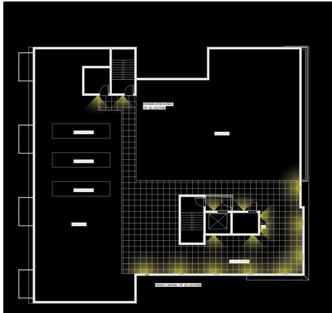
A Roof level lighting plan
