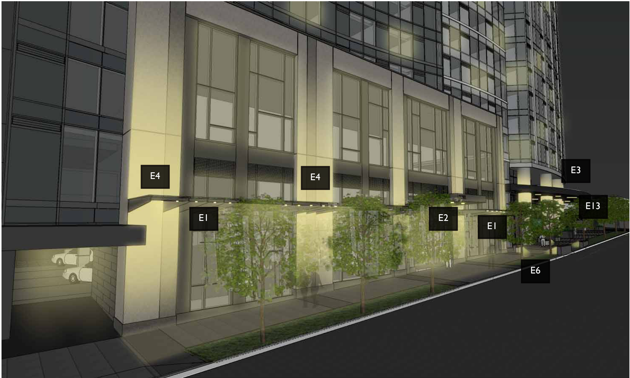
E4 LED LINEAR UPLIGHT AND DOWNLIGHT TWO LINEAR LIGHTS ACCENT THE COLUMNS WITH UPLIGHT AND DOWNLIGHT FROM NICHES WITHIN THE CANOPY.
