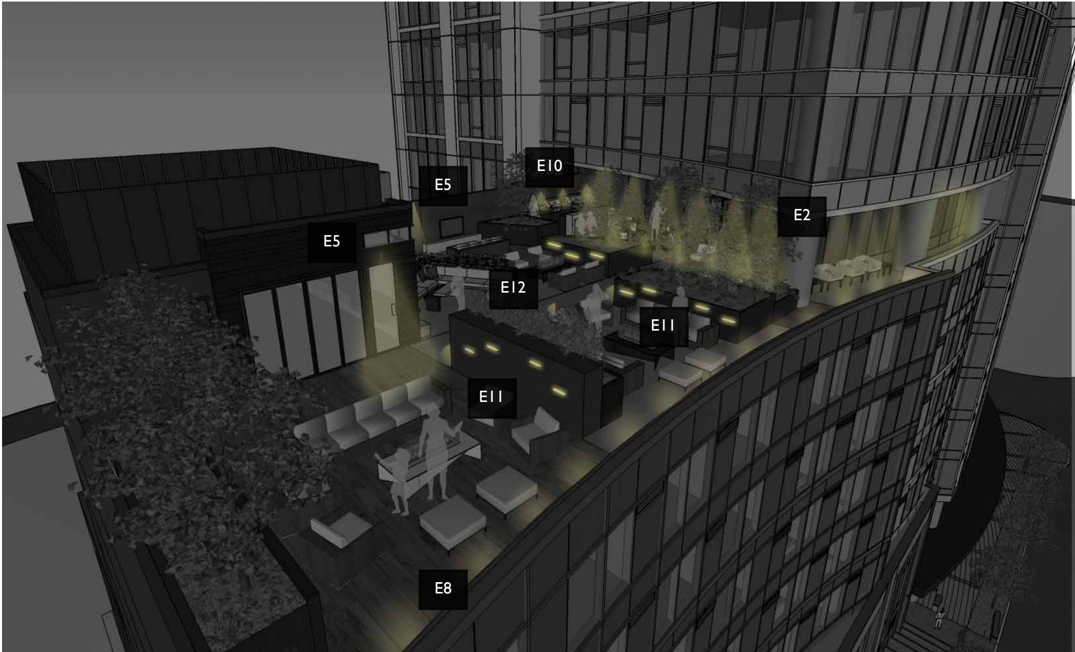
E10 LED TABLE MOUNTED ADJUSTABLE BBQ LIGHT ADJUSTABLE TABLE LIGHTS PROVIDE TASK LIGHTING AT EACH BBQ GRILL.
