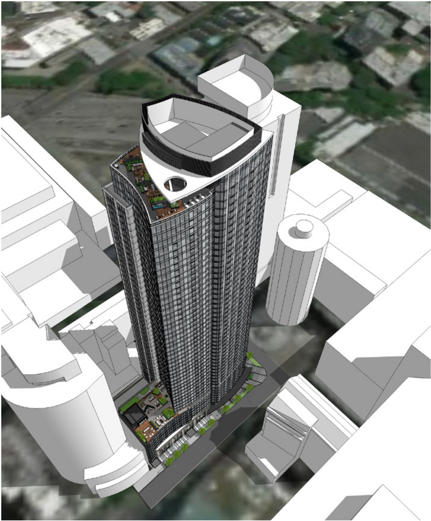
The 8th Ave tower facade is broken down into two main elements, the “A” wall and the “B” wall which are separated by a gasket that runs the length of the tower in order to improve the perception of slenderness and enhance the tower proportions.
