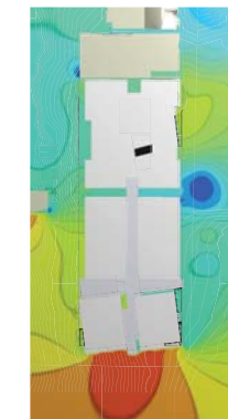
average wind pressure diagram measuring affect of exterior circulation spine to create a protected environment
