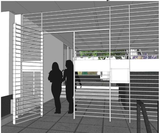
Main Entry Gate with Call Box - white steel flat bar at 4" o.c.
