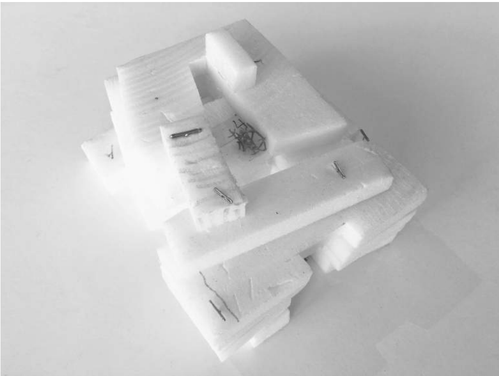
SITE MODEL A series of study models explored the network of sidewalk-connected passageways, a central courtyard, and rooftop amenity spaces.
