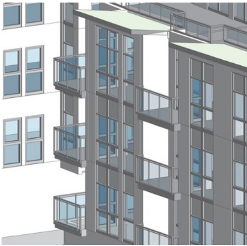
DC-4: Vinyl window with glass spandrel
