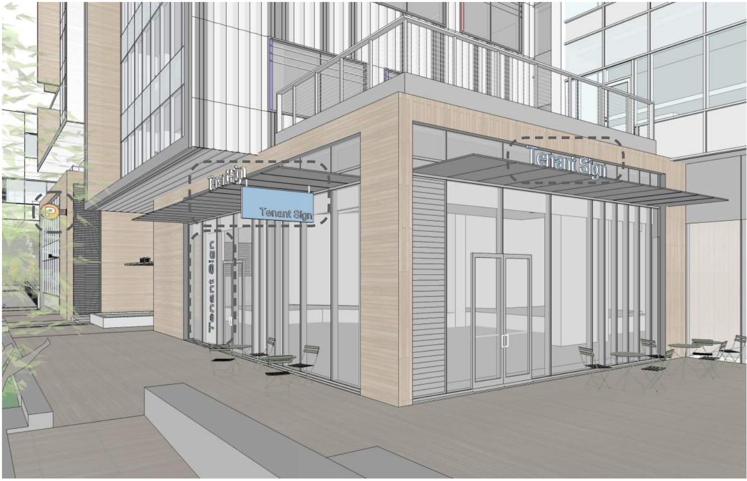
Description: Hung from canopy or wall adhered. Three-dimensional relief letters in stainless steel or powder-coated metal. (Note: final retail signage is subject to retailer's requirements and will be reviewed by owner for consistency with building design).
