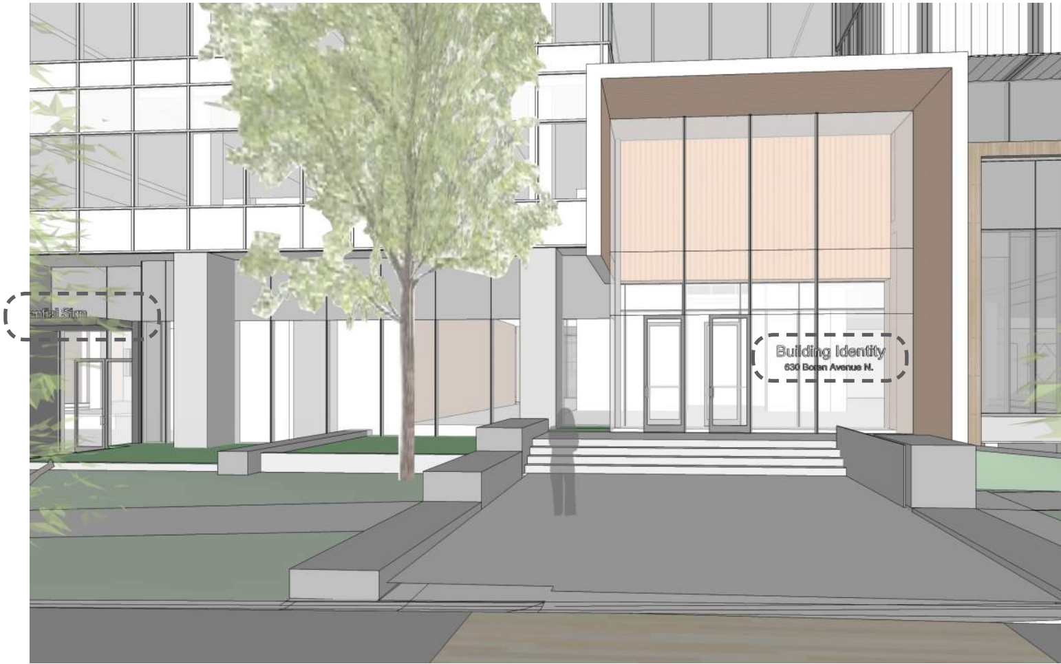
Description: Pin-mounted to facade or landscape monument. Three-dimensional relief letters in stainless steel, powder-coated metal or illuminated channel letters. (Note: final commercial building identity is subject to tenant's requirements and will be reviewed by owner for consistency with building design).
