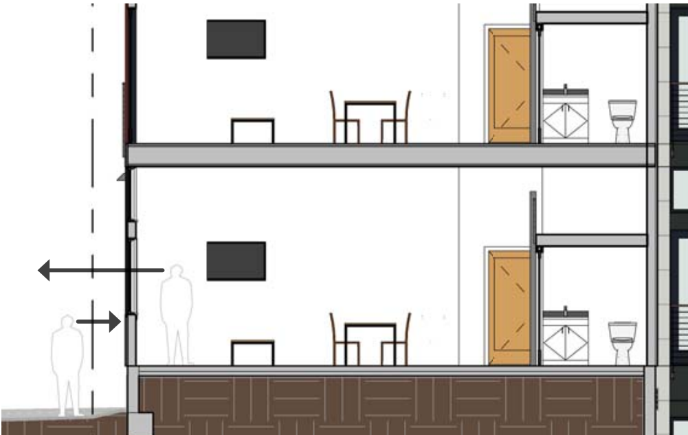
Section at unit: Casement windows are installed higher to block views from the alley.
