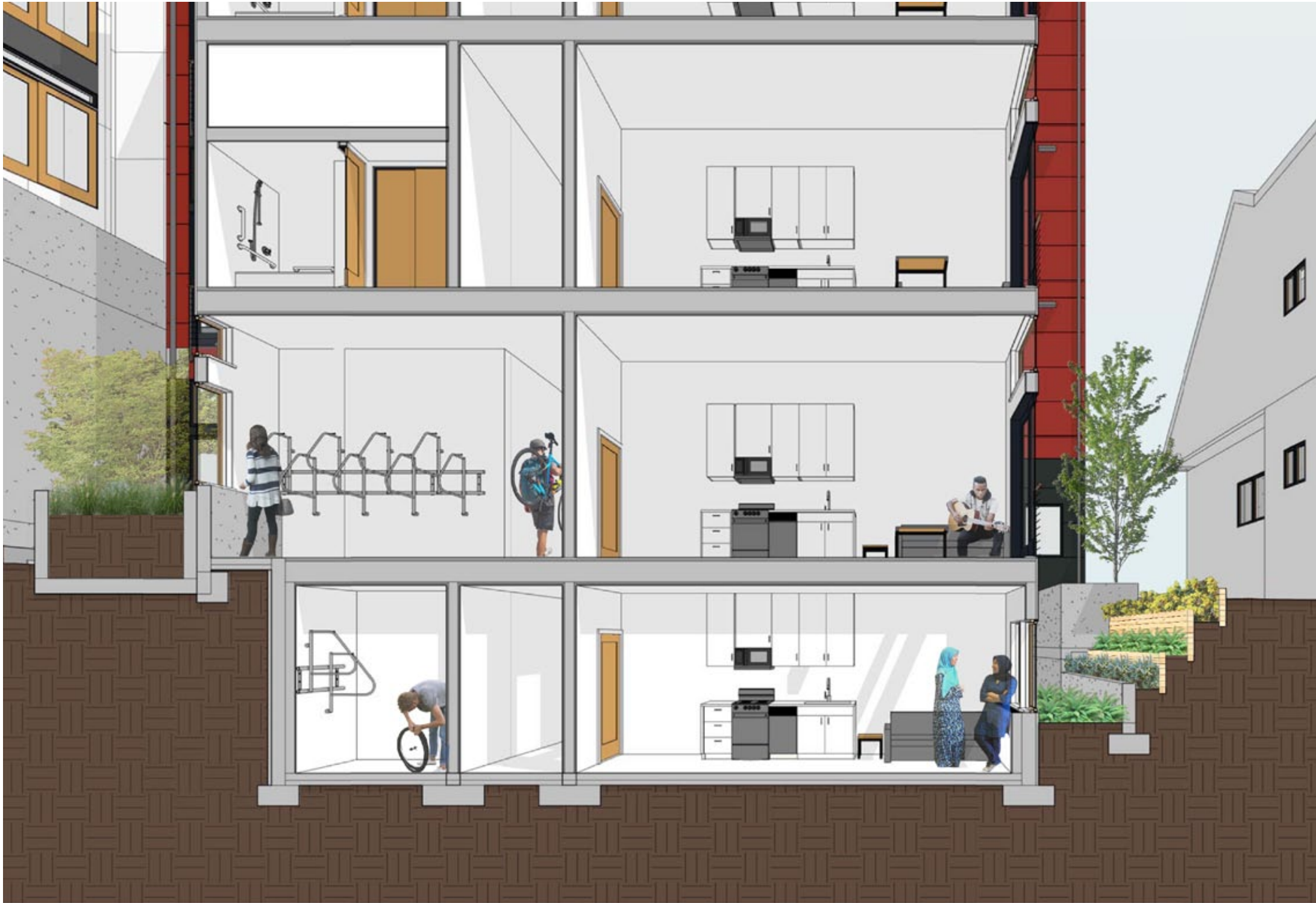
Transverse section perspective looking east: The terraced landscaping provides more light and air to the window wells of the basement units.
