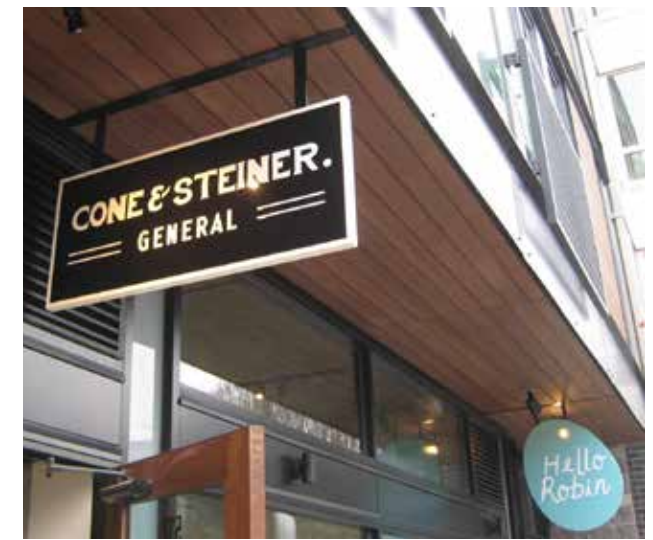
Externally-illuminated under-canopy blade sign
