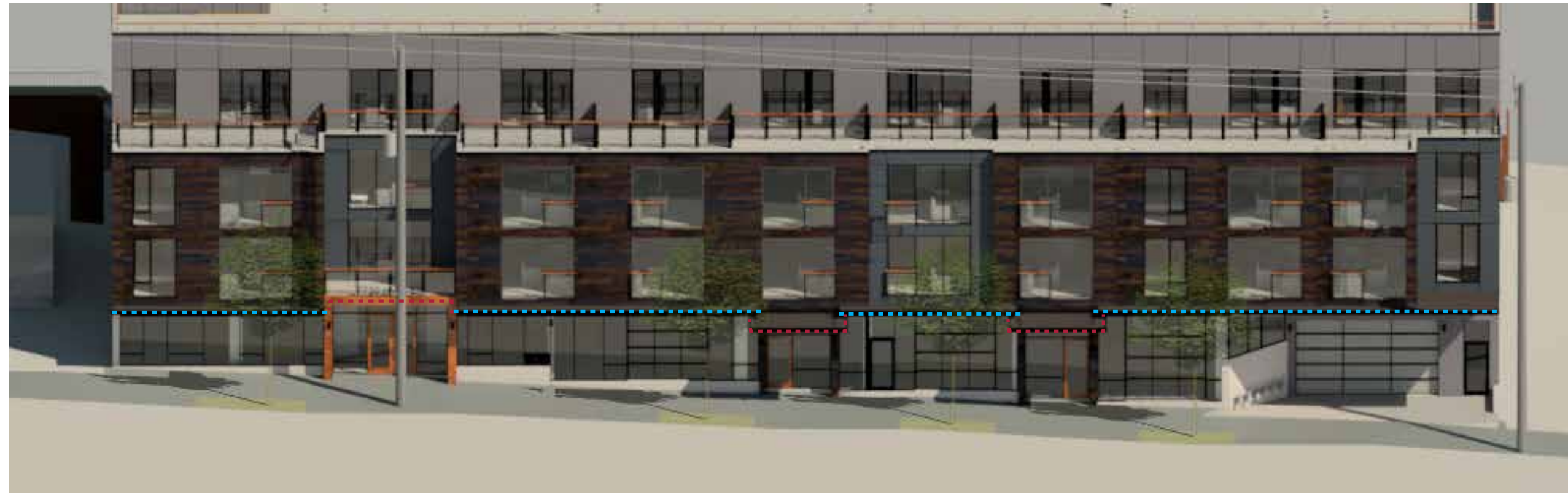
^ proposed design (with departure) from 15th Ave NW. Canopy design highlights building entry points and aligns with facade modulation
