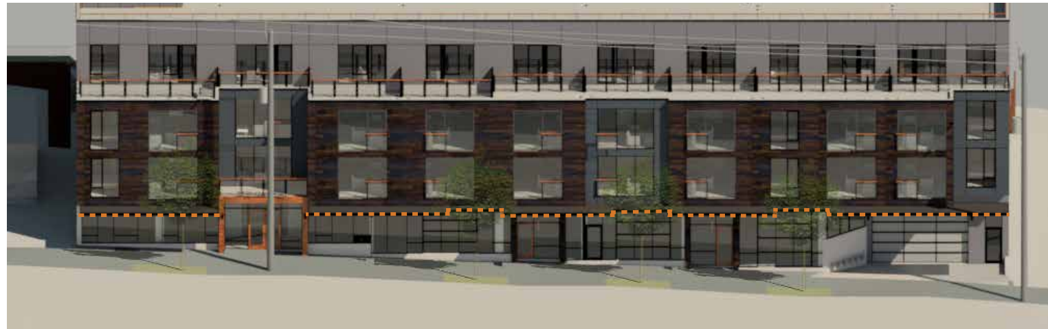
^ Code-compliant design with notched canopy at street tree locations. Canopy has no relationship to entries or facade composition
