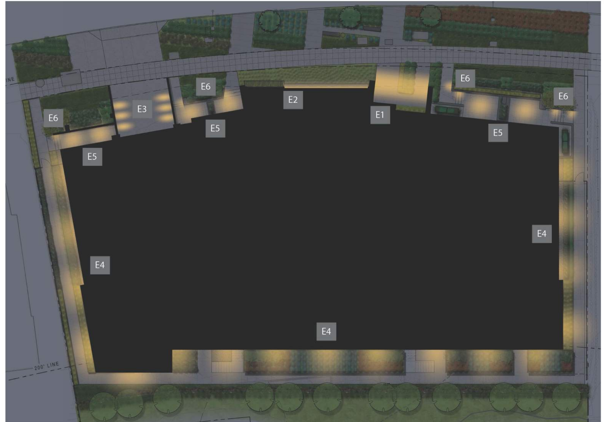
E5 SURFACE MOUNT LED DOWNLIGHT LED DOWNLIGHT SURFACE MOUNTED OVER EACH UNIT PATIO
