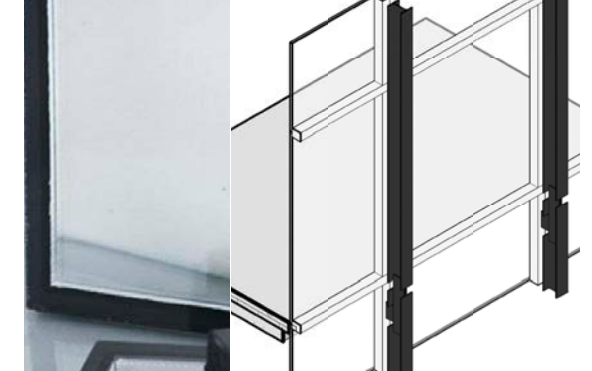
CW-2 4" WIDE ALUMINUM CURTAIN WALL SYSTEM SUPPORTED BY EXTERIOR STEEL
