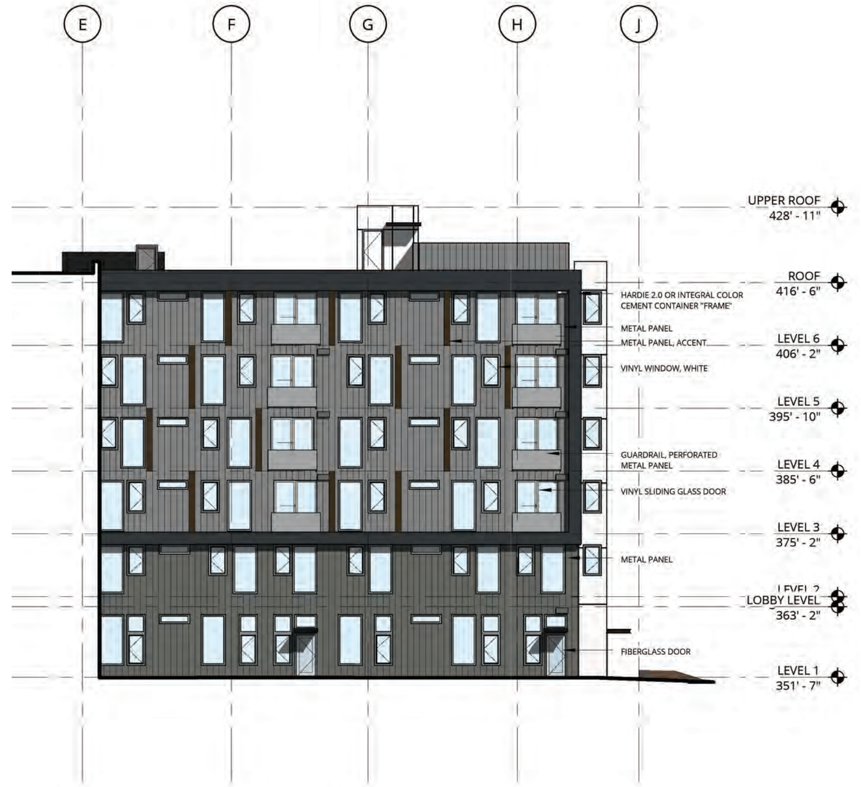
COURTYARD EAST ELEVATION
