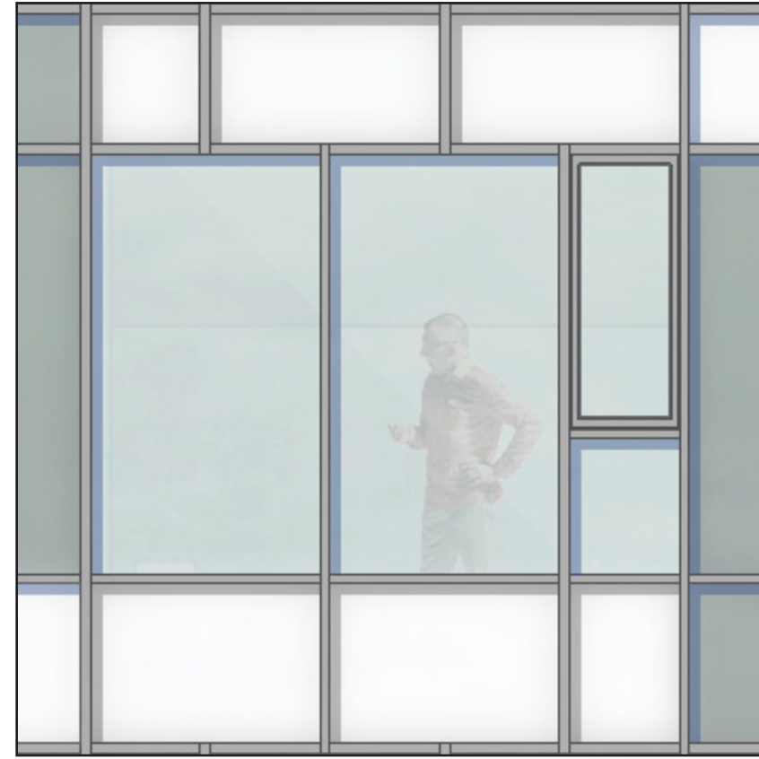
Enlarged East Elevation Window Wall Modules
