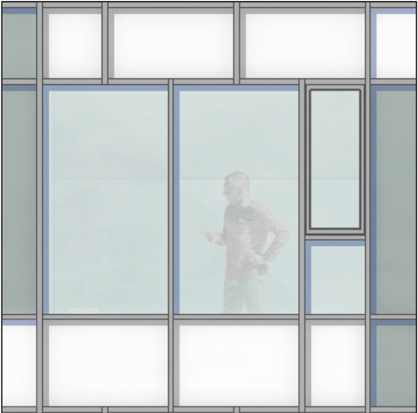
Enlarged East Elevation Window Wall Modules
