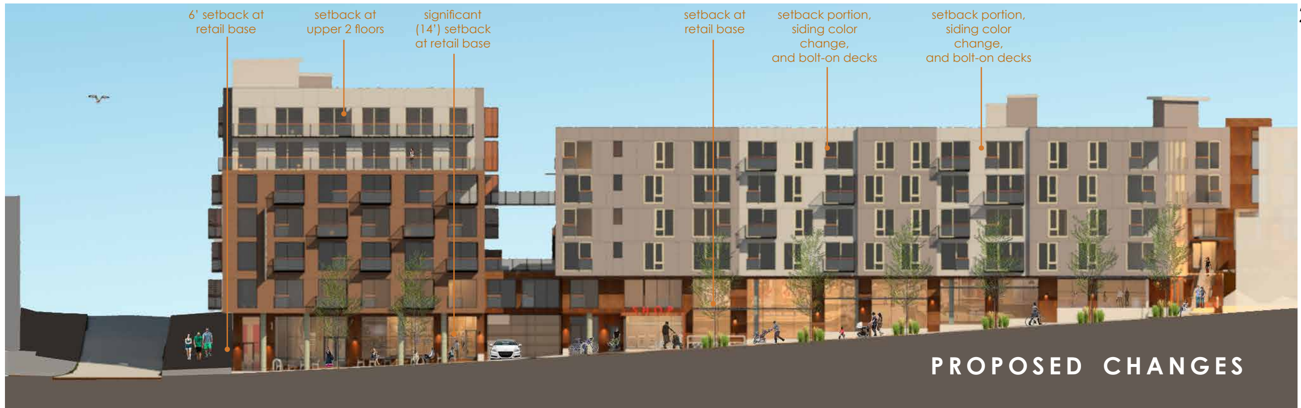
Facade Modulation along S Alaska St (North Elevation)
