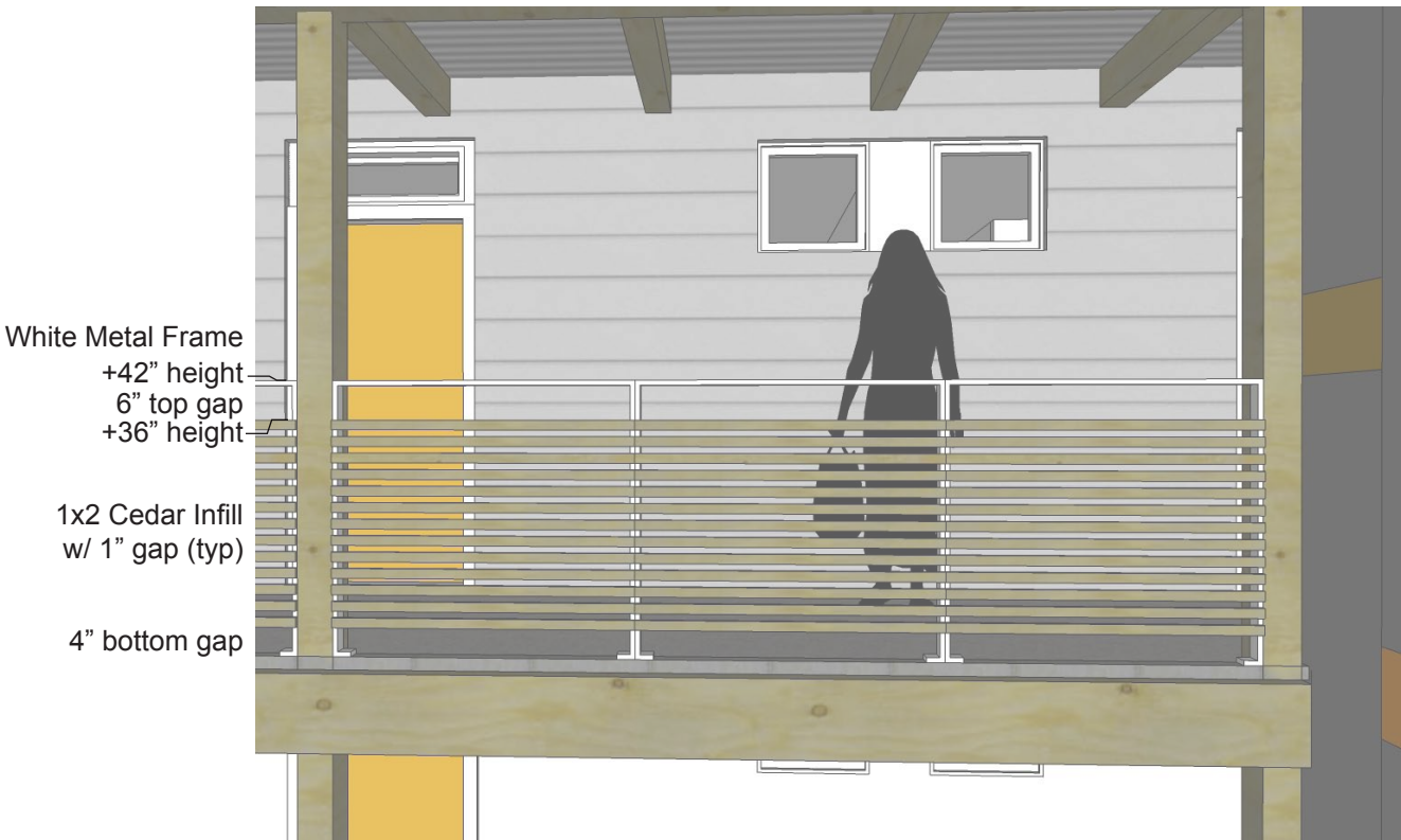
Typical Railing Detail
