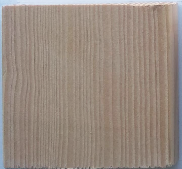
W-1 WOOD STRUCTURE DOUGLAS / HEMLOCK FIR (PER STRUCT) CLEAR COAT FINISH
