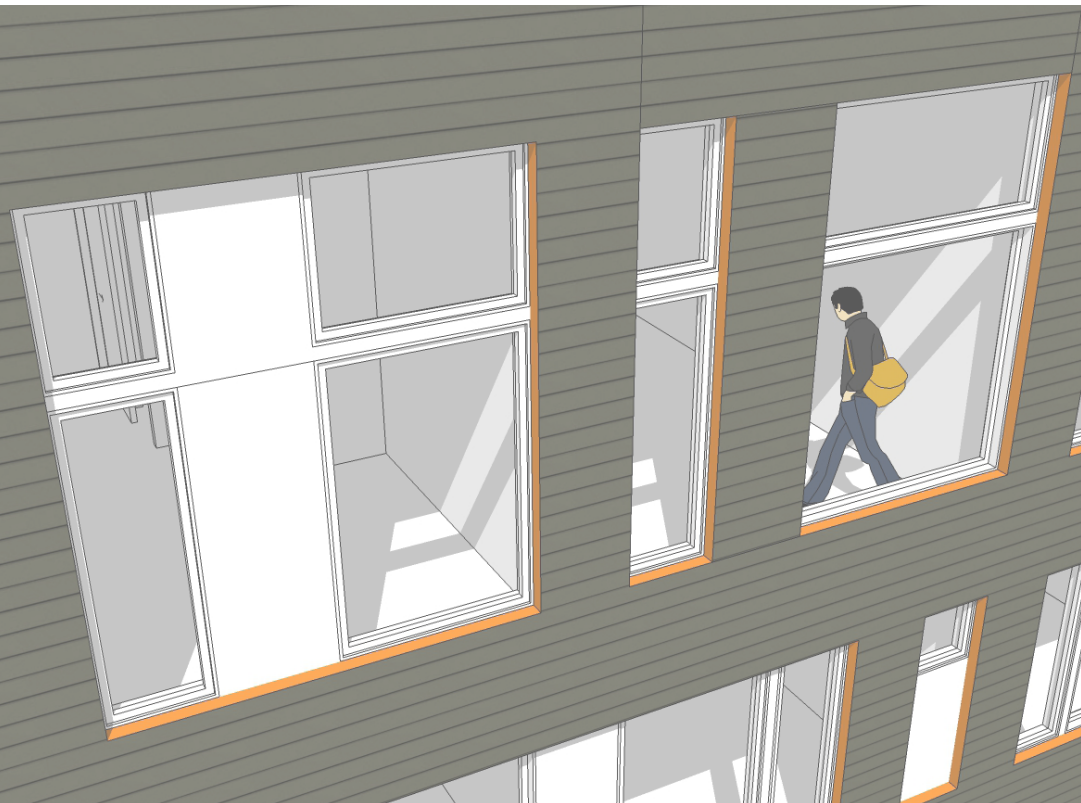
Windows inset 4" from exterior face to add depth to face with accent trim to articulate openings
