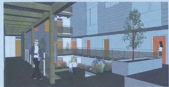
W-1 WOOD STRUCTURE DOUGLAS / HEMLOCK FIR (PER STRUCT) CLEAR COAT FINISH
