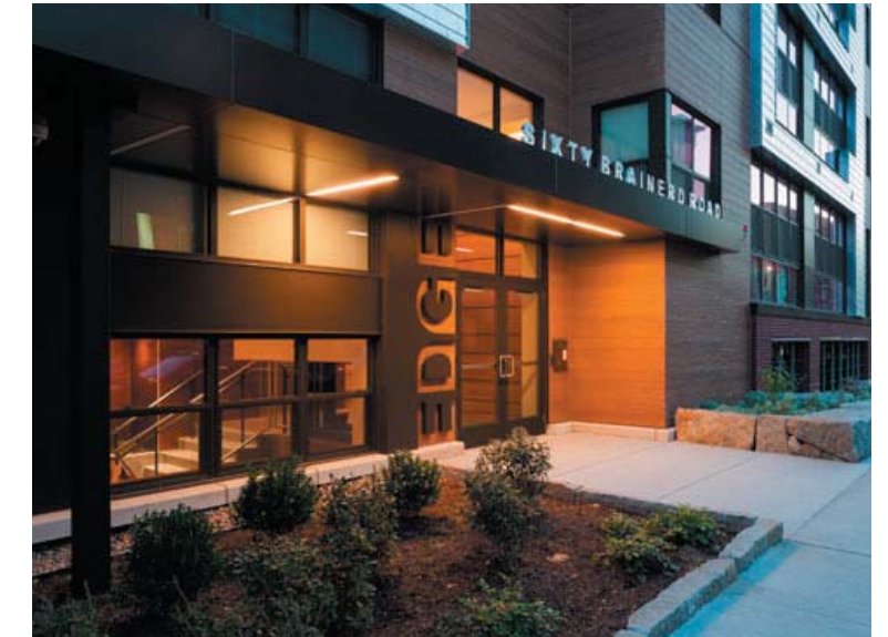
RESIDENTIAL ENTRY: RECESSED FULLY GLAZED STOREFRONT ENTRY WITH AN EXTENDED AWNING ENGAGING THE PATHWAY APPROACH
