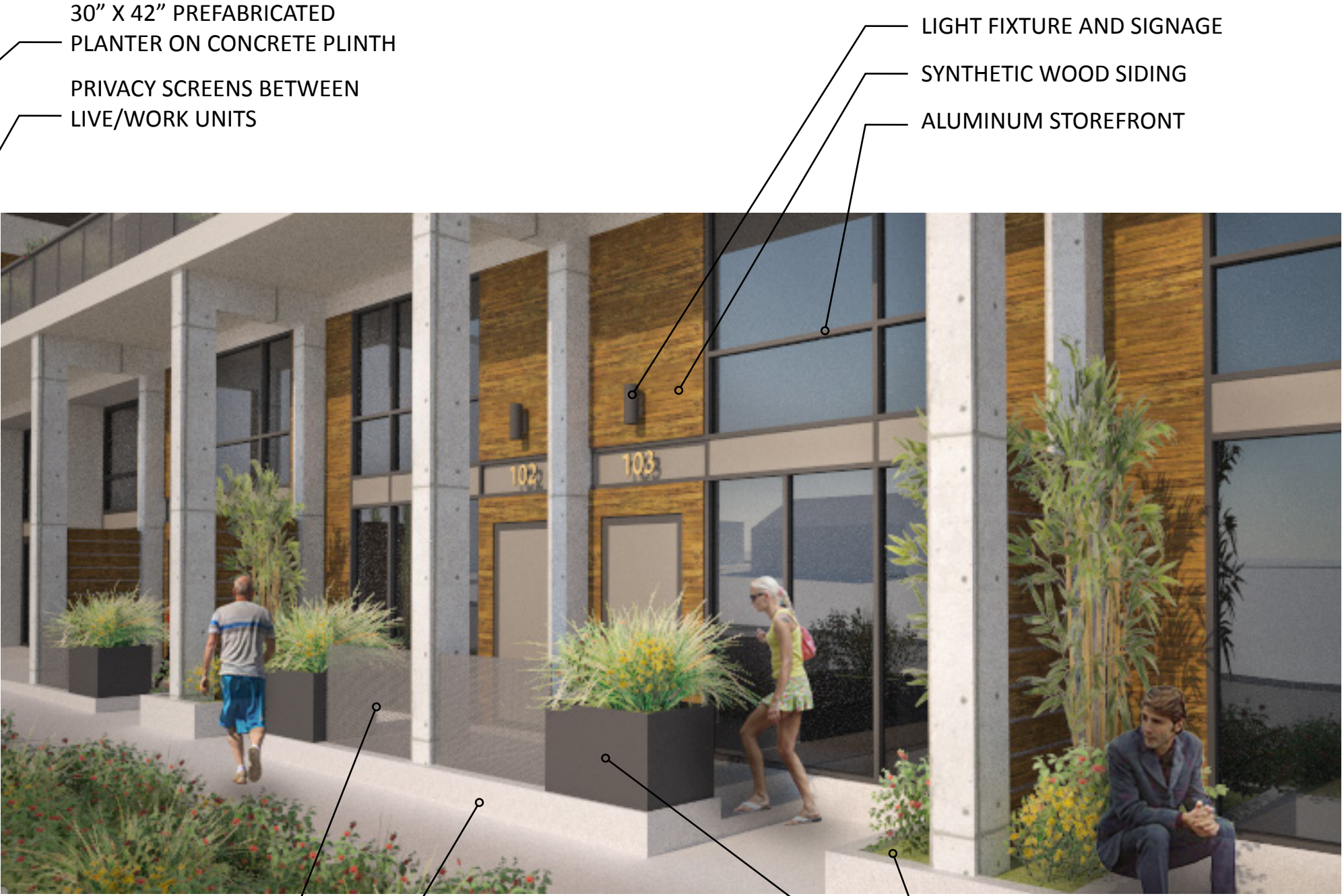
DECORATIVE METAL SCREEN CAST-IN-PLACE CONCRETE STOOP
