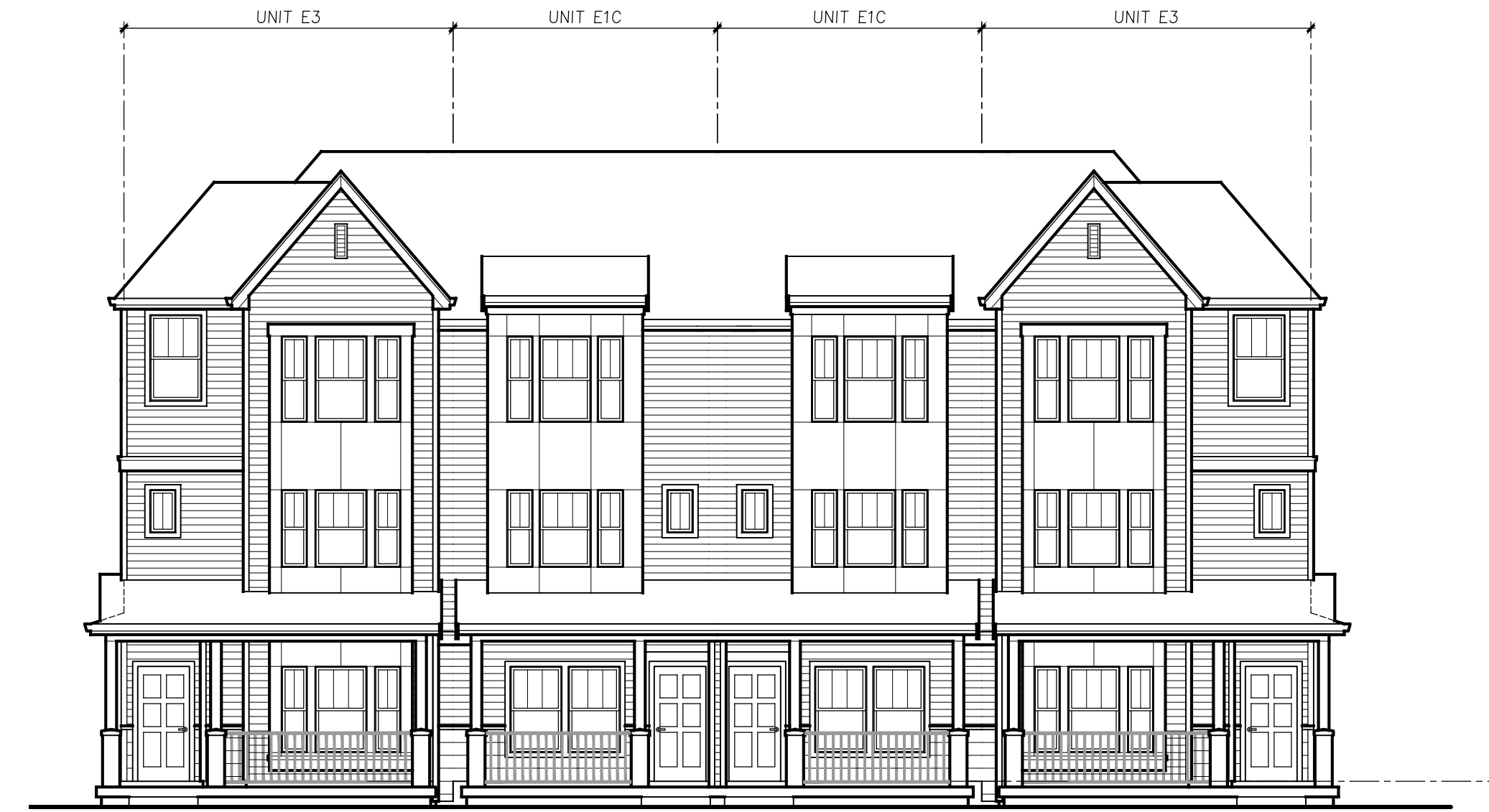
REAR LOADED 4-PLEX TOWNHOME FRONT ELEVATION 1/8" = 1'-0" BUILDINGS 6 & 7
