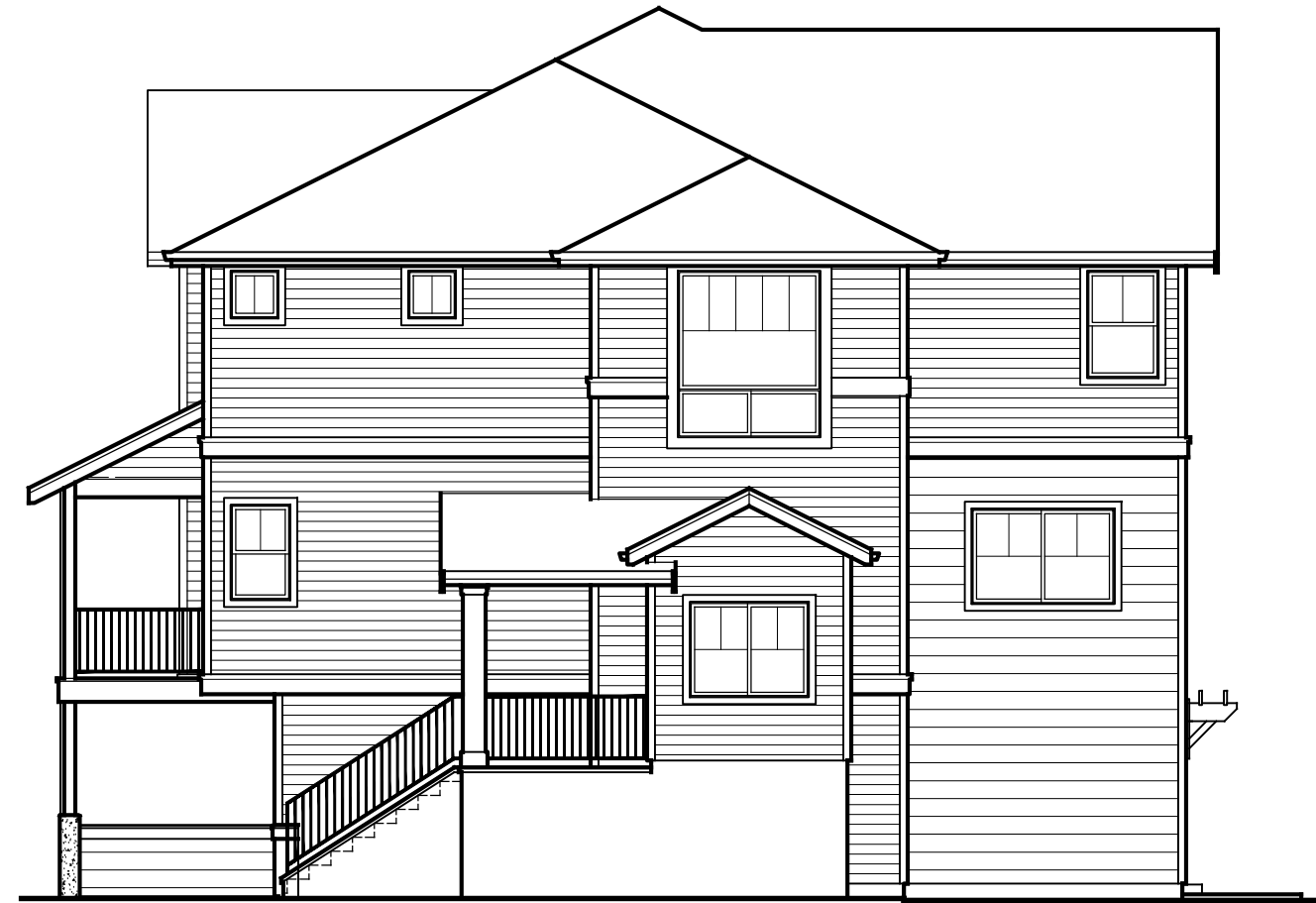
FRONT LOADED 5-PLEX TOWNHOME LEFT ELEVATION 1/8" = 1'-0" BUILDINGS 1 & 10
