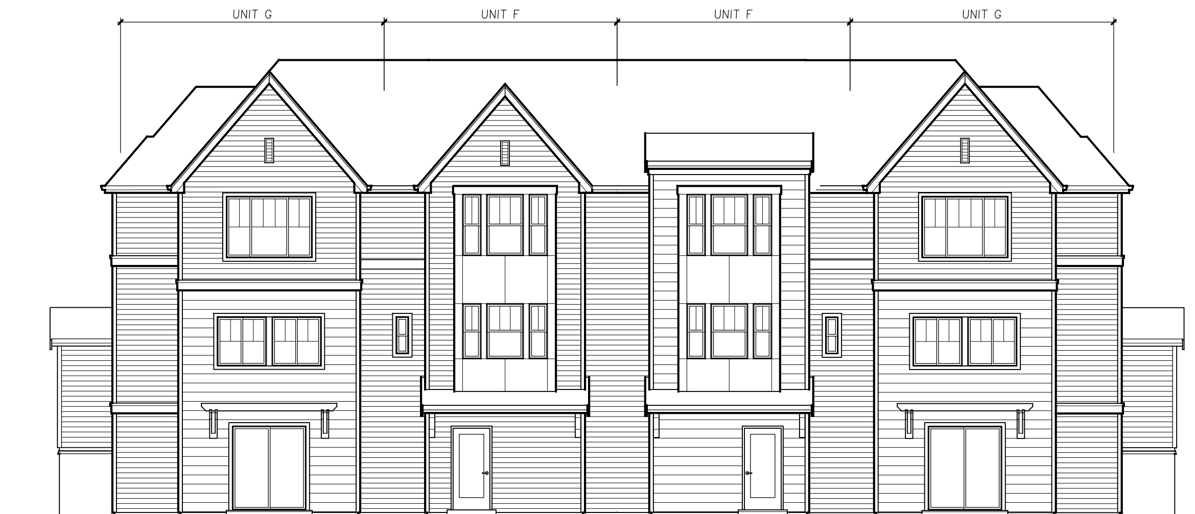
FRONT LOADED 4-PLEX TOWNHOME REAR ELEVATION 1/8" = 1'-0" BUILDINGS 4, 5 & 8
