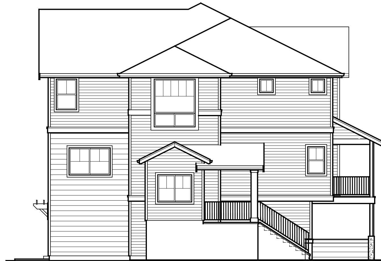
FRONT LOADED 5-PLEX TOWNHOME RIGHT ELEVATION 1/8" = 1'-0" BUILDINGS 1 & 10
