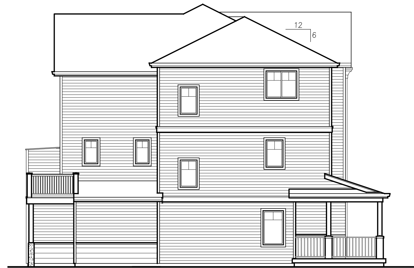
REAR LOADED 6-PLEX TOWNHOME LEFT ELEVATION 1/8" = 1'-0" BUILDINGS 2 & 9
