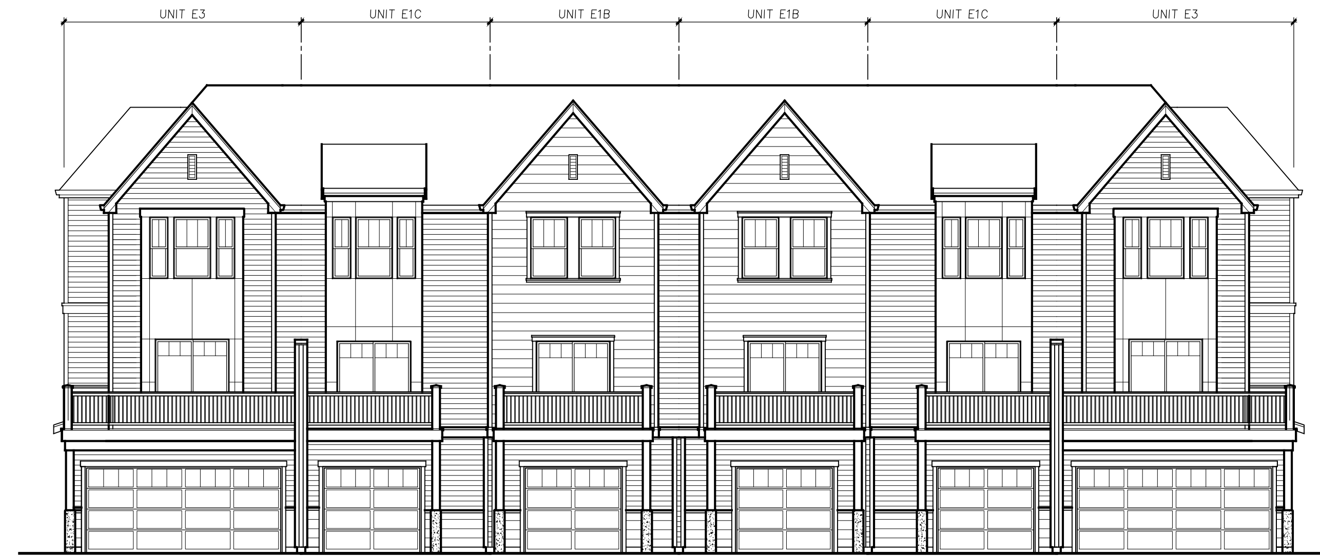
REAR LOADED 6-PLEX TOWNHOME REAR ELEVATION 1/8" = 1'-0" BUILDINGS 2 & 9
