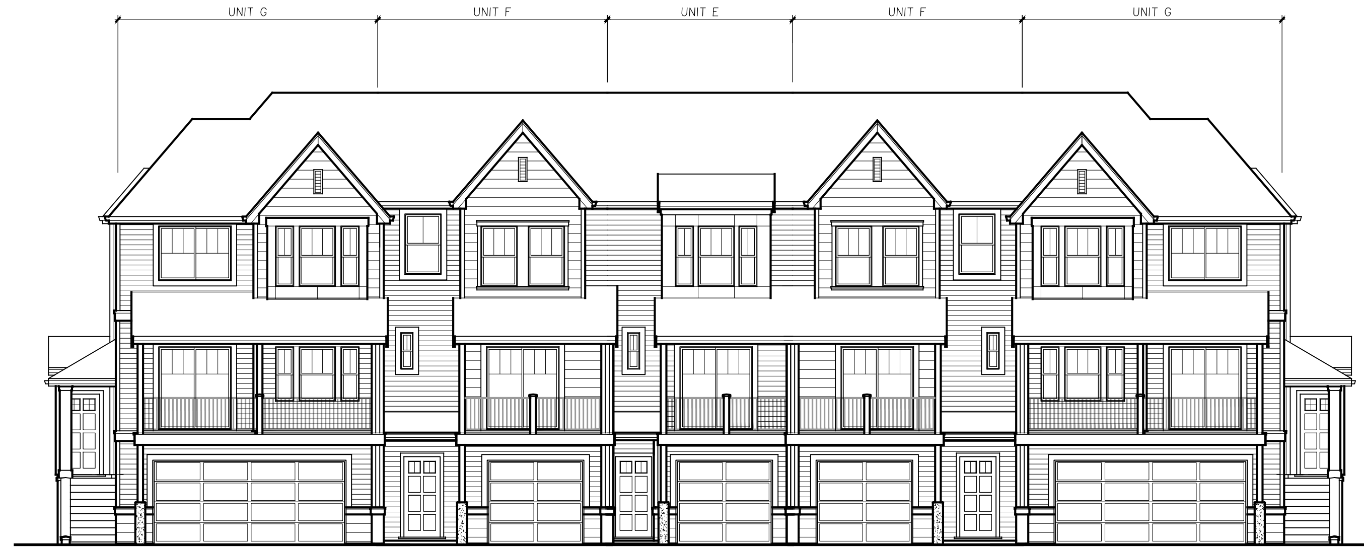
FRONT LOADED 5-PLEX TOWNHOME FRONT ELEVATION 1/8" = 1'-0" BUILDINGS 1 & 10
