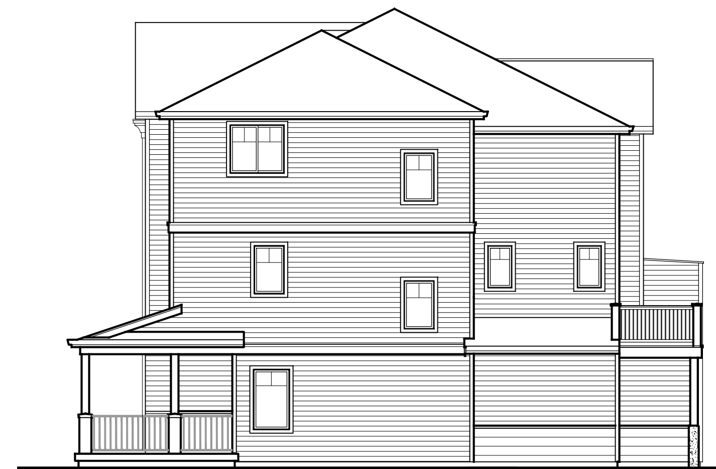
REAR LOADED 4-PLEX TOWNHOME RIGHT ELEVATION 1/8" = 1'-0" BUILDINGS 6 & 7
