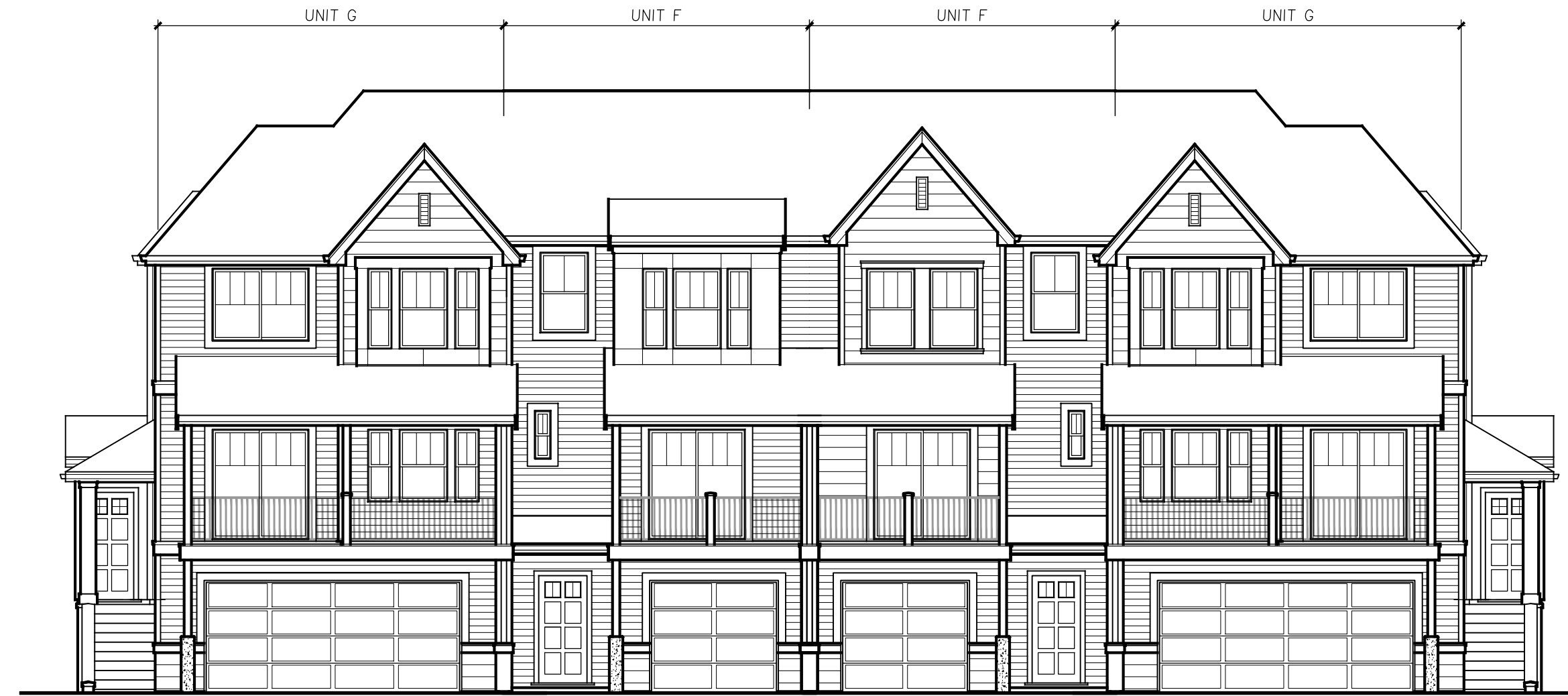
FRONT LOADED 4-PLEX TOWNHOME FRONT ELEVATION 1/8" = 1'-0" BUILDINGS 4, 5 & 8
