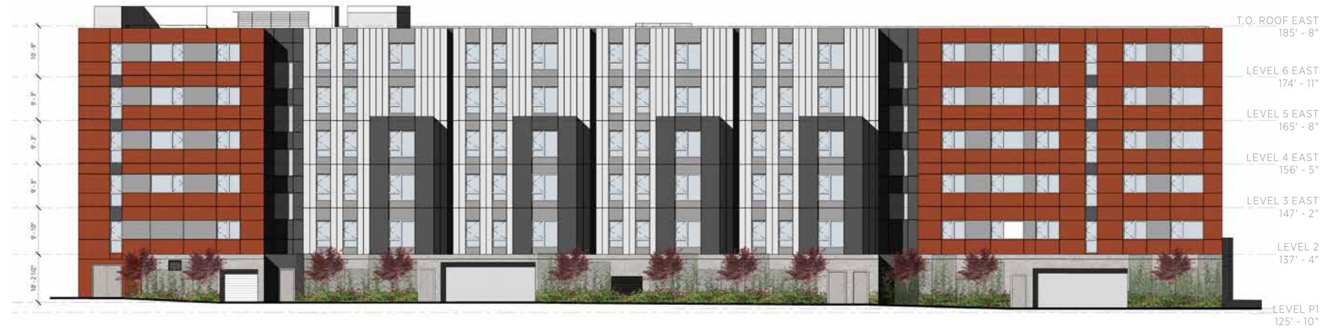
EAST ELEVATION: LOWER PARAPETS (ALTERNATIVE)
