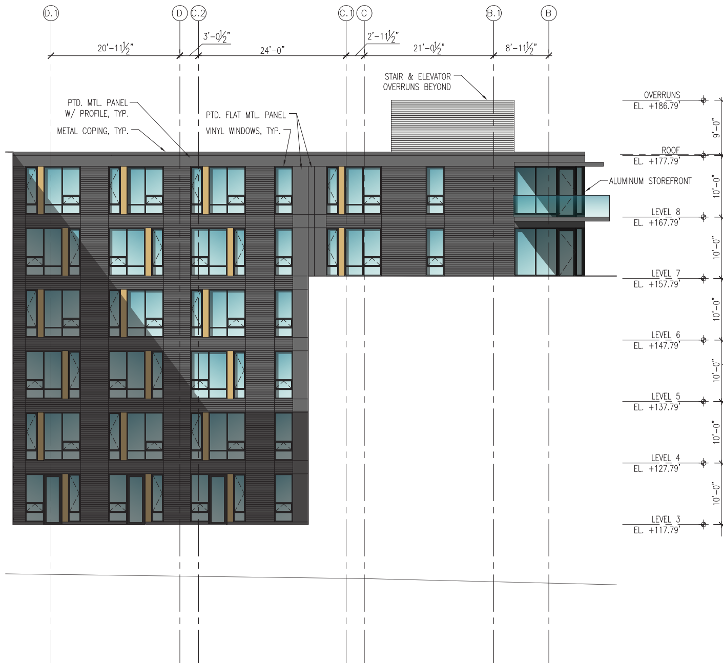
1 EAST ELEVATION SCALE: 1/8"=1'-0"
