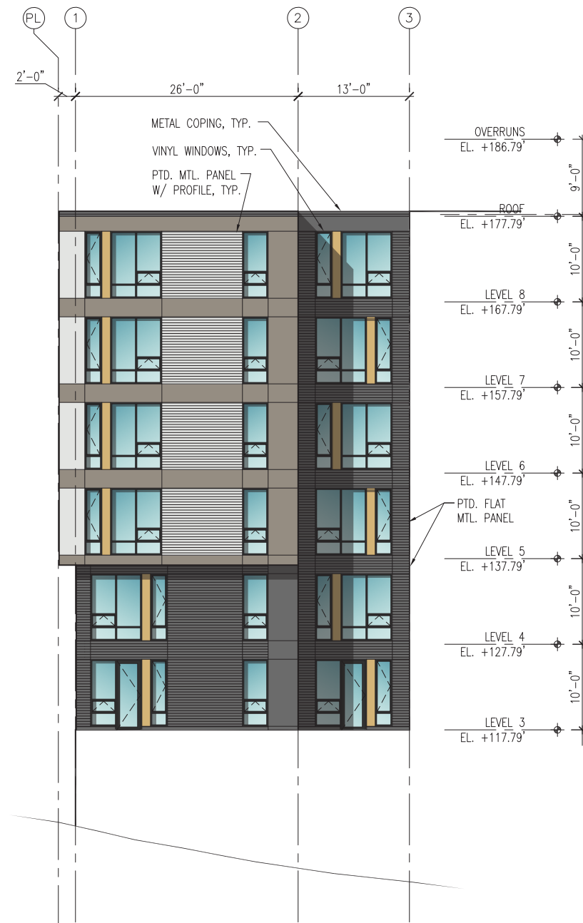
2 SOUTH ELEVATION SCALE: 1/8"=1'-0"
