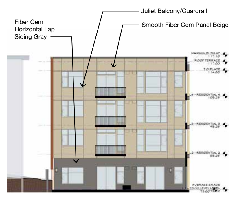
NORTH COURTYARD ELEVATION - VIEW NORTH
