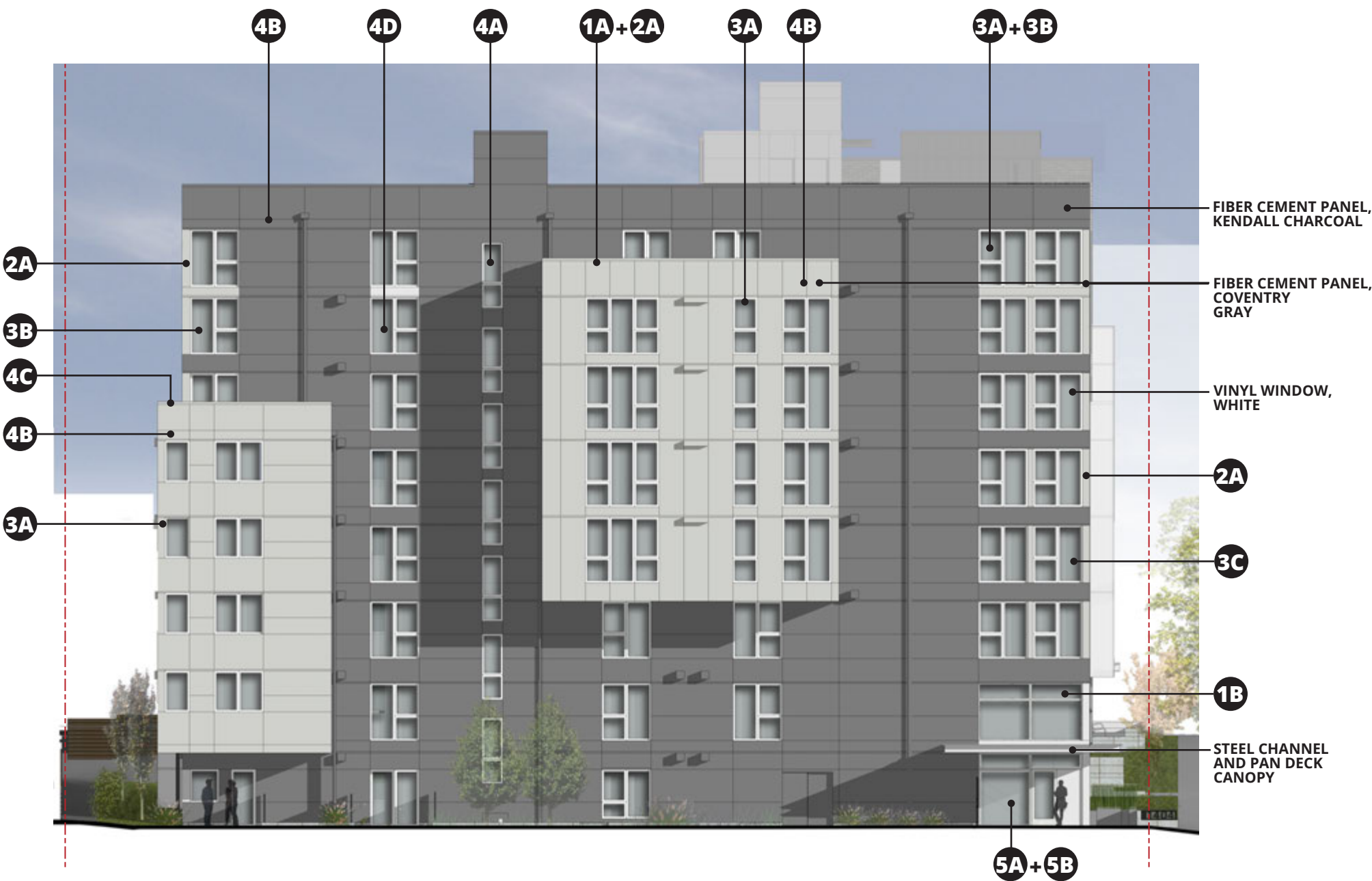
ELEVATION ALONG NORTH PROPERTY LINE: SIMPLE SCHEME
