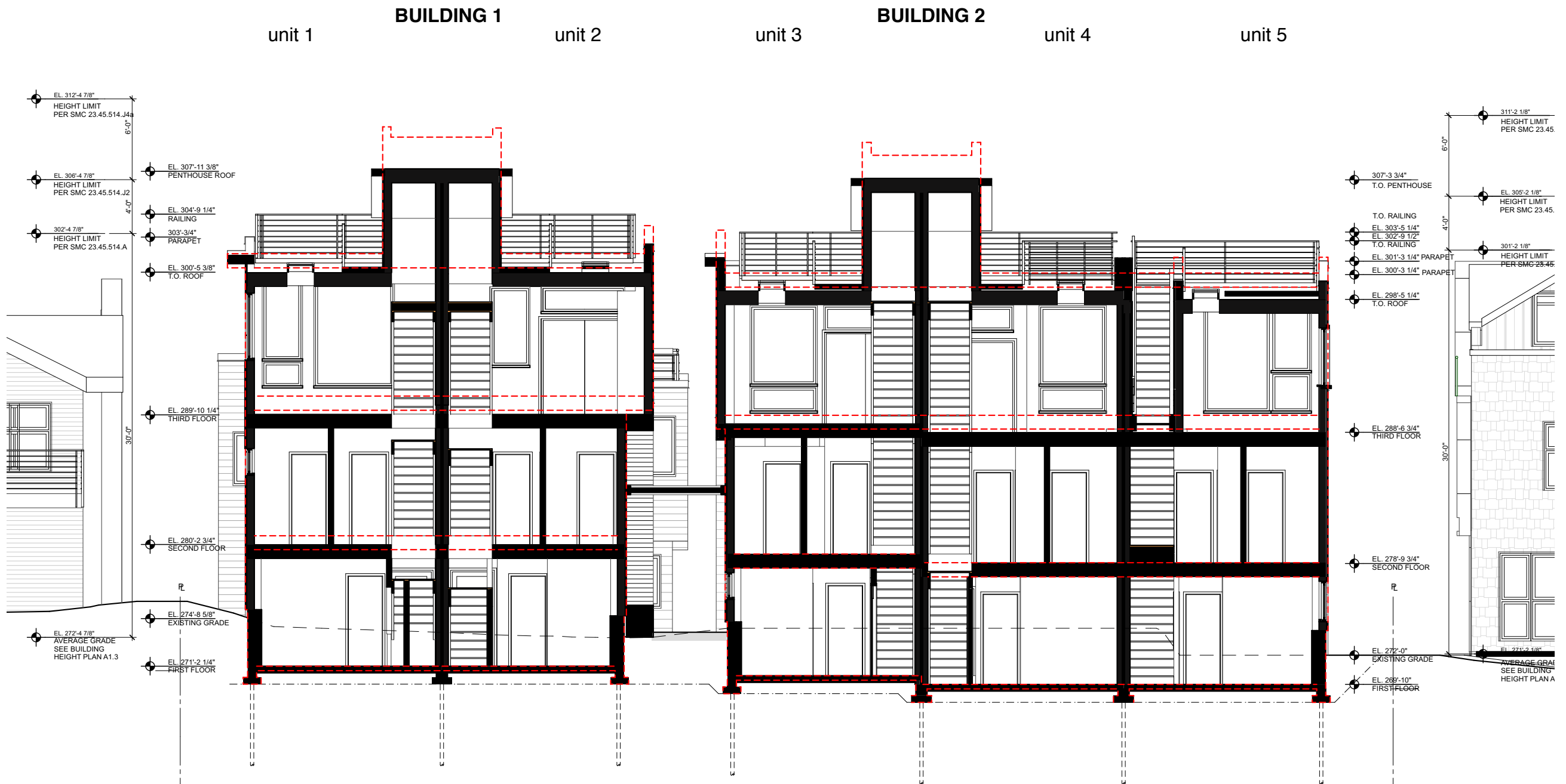
TRANSVERSE SECTION THROUGH BUILDINGS 1 AND 2
