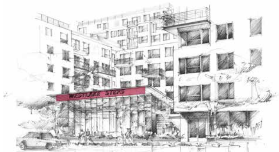
Dimensional letter-forms pin mounted from below soffit overhead of glass structure.
