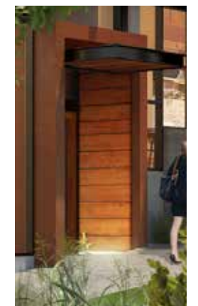
Wall-wash uplight @ entry portal interior
