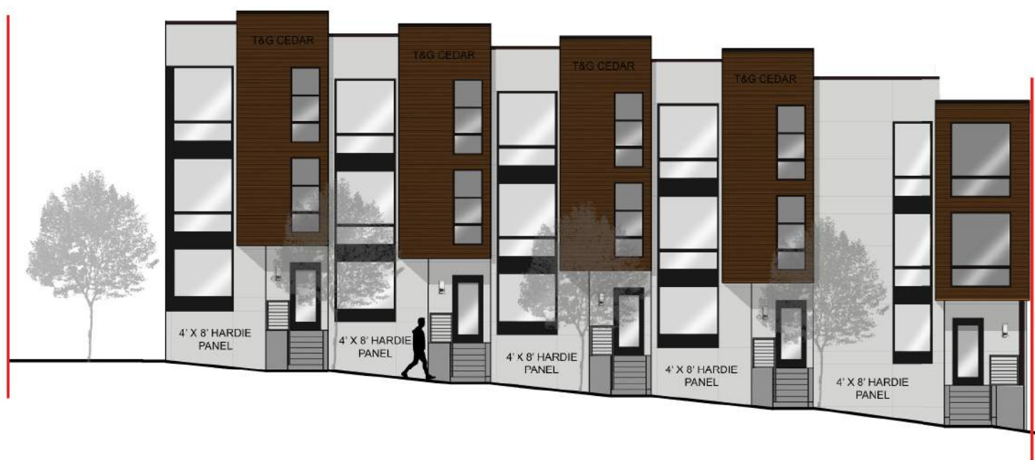
○ BUILDING 2 - EAST ELEVATION NTS
