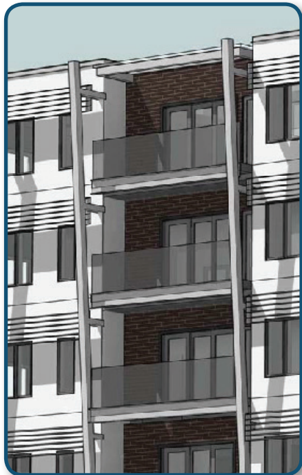
detail: sunshades and decks in galvanized steel
