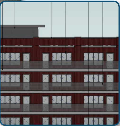
black window frames, AEP Span box rib metal in Cool Colonial Red
