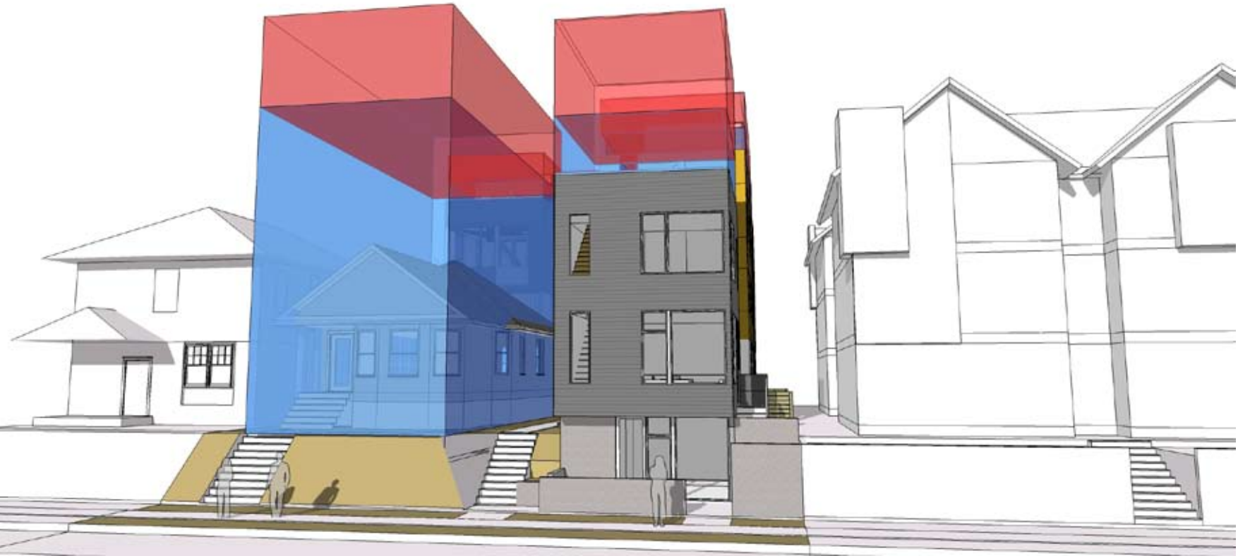
Blue shaded area - max bulk as townhouse structure (30' base height plus bonus) Red shaded area - max bulk as an apartment structure (40' base height plus bonus)
