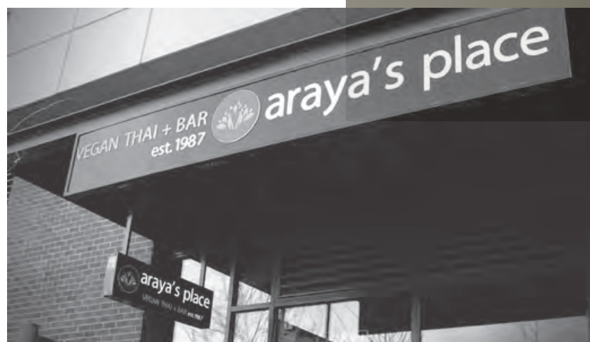
DOUBLE SIDED UNDER MOUNTED CANOPY BLADE SIGN + TOP MOUNTED CANOPY BOX SIGN
