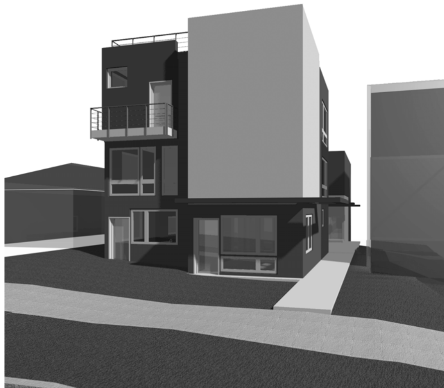
Design Evolution •Deck projection counts toward facade length •Awning at ground level for interest and scale
