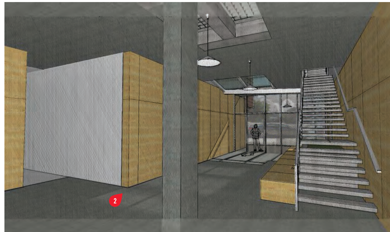
3D SKETCH OF OPEN AIR RESIDENTIAL ENTRY SHOWING CANTILEVERED CONCRETE STAIR AT L1
