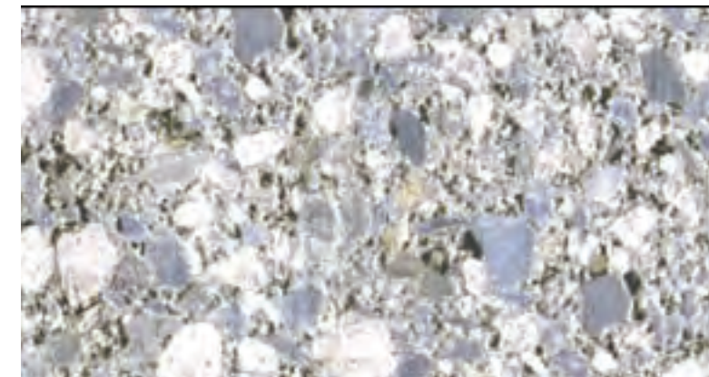
MASONRY GROUND FACE CMU
