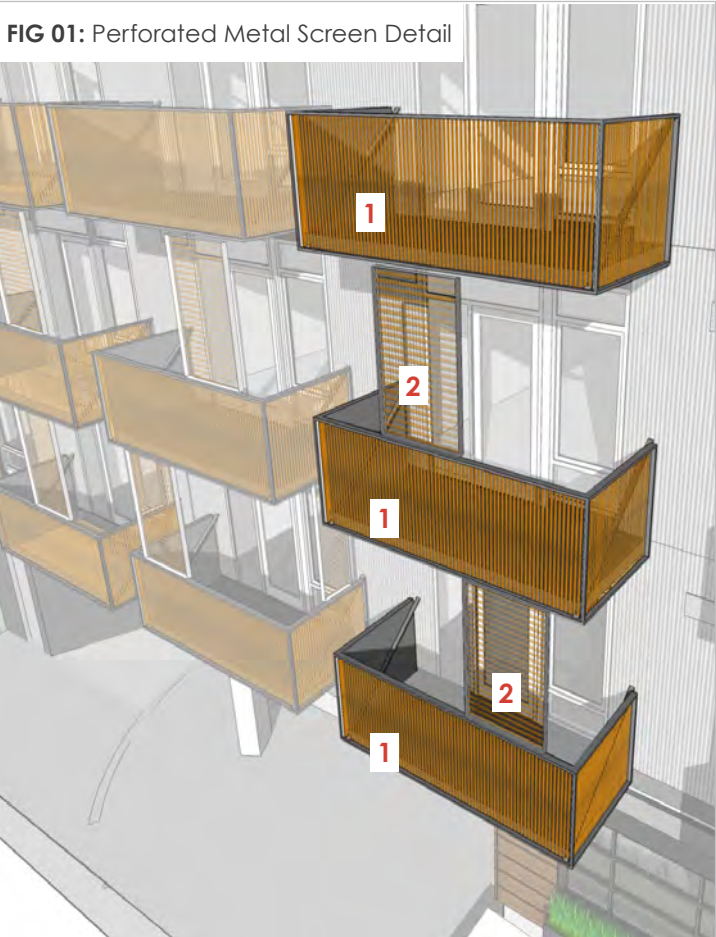
1. Guardrail: Corrugated Perforated Metal Panel Supported By Welded Steel Frame
