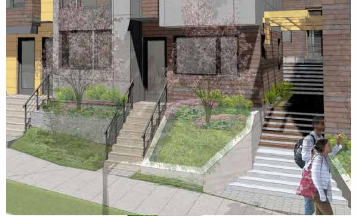
Proposed project: terraced planters transition to the sidewalk to a maximum height of 5'-2". Recessed entries create a rhythm and provide privacy.
