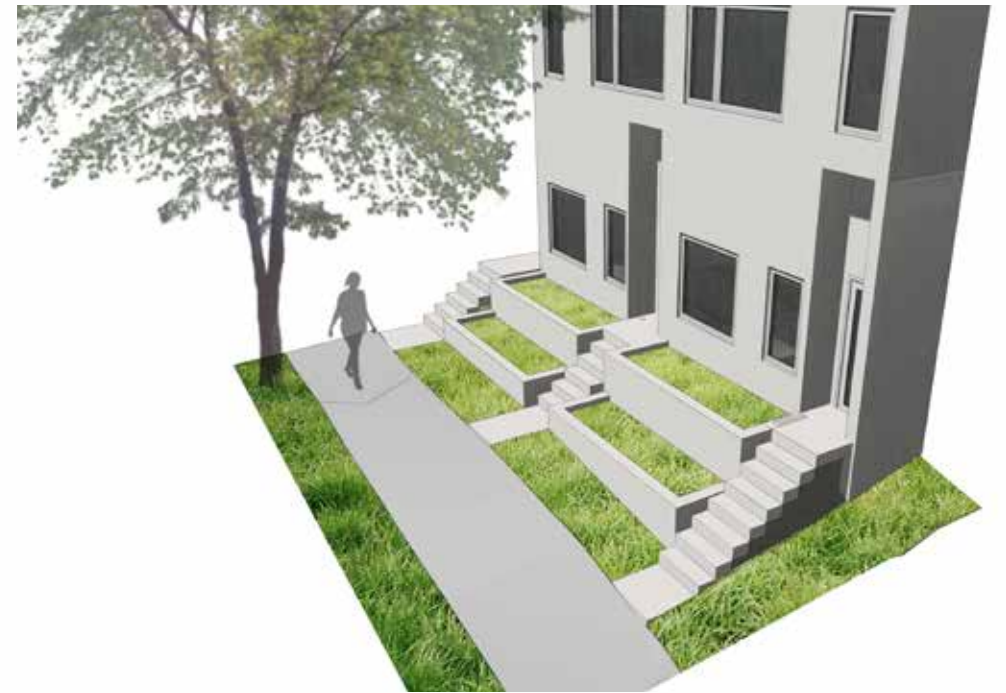
Terraced planters transition to the sidewalk to a maximum height of 5'-2". Recessed entries create a rhythm and provide privacy.
