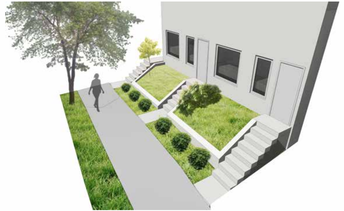
A sloped retaining wall transitions from a minimum height of 6" to the top of the landing at 5'-2".
