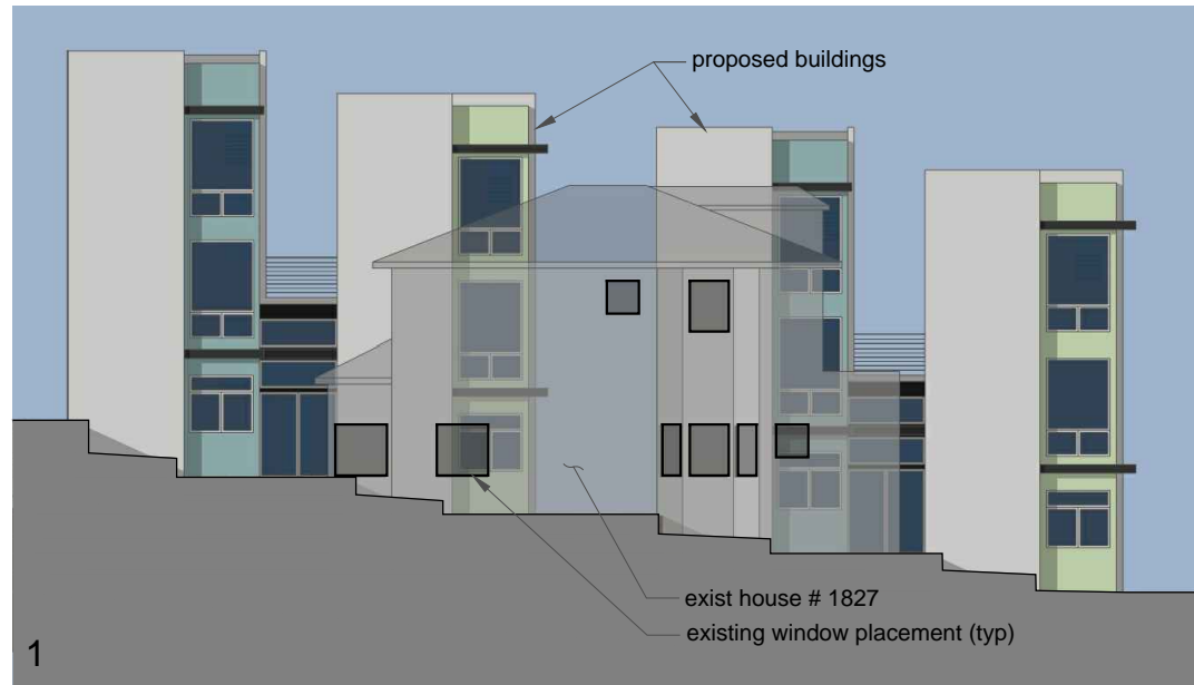
1 window alignment at south property line
