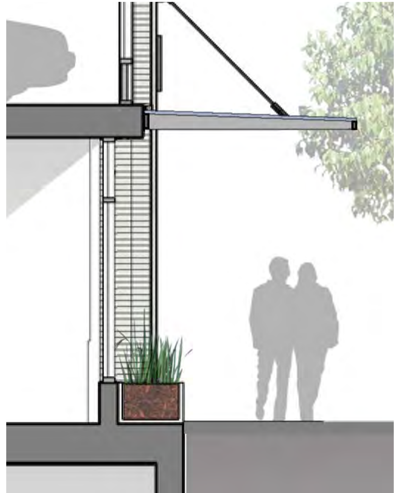
SECTION: REVISED TRANSPARENT CANOPY AT STOREFRONT GLAZING
