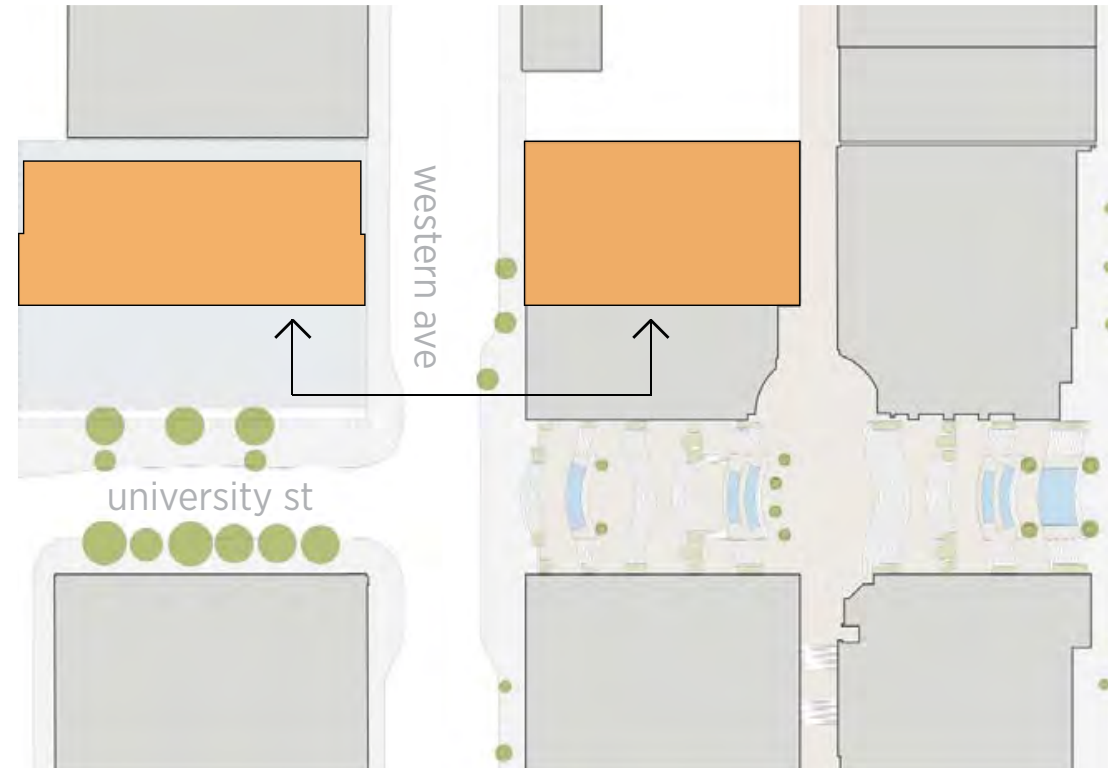
Proposed massing showing impact of green street upper level setback and view corridor setback. Double setback does not meet Design Guidelines A-1, B-1, B-3, B-4
