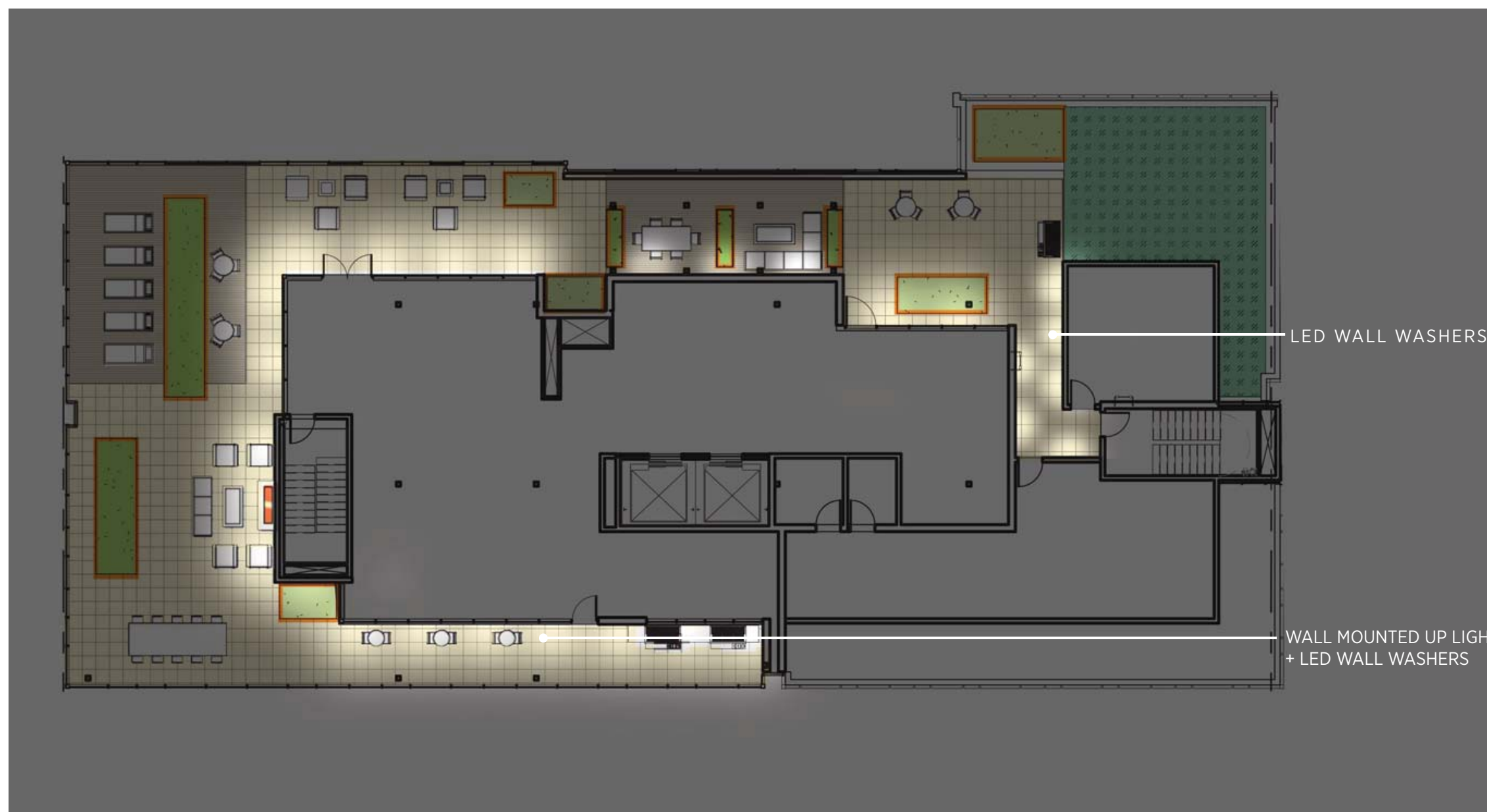
ROOF LEVEL EXTERIOR LIGHTING PLAN
