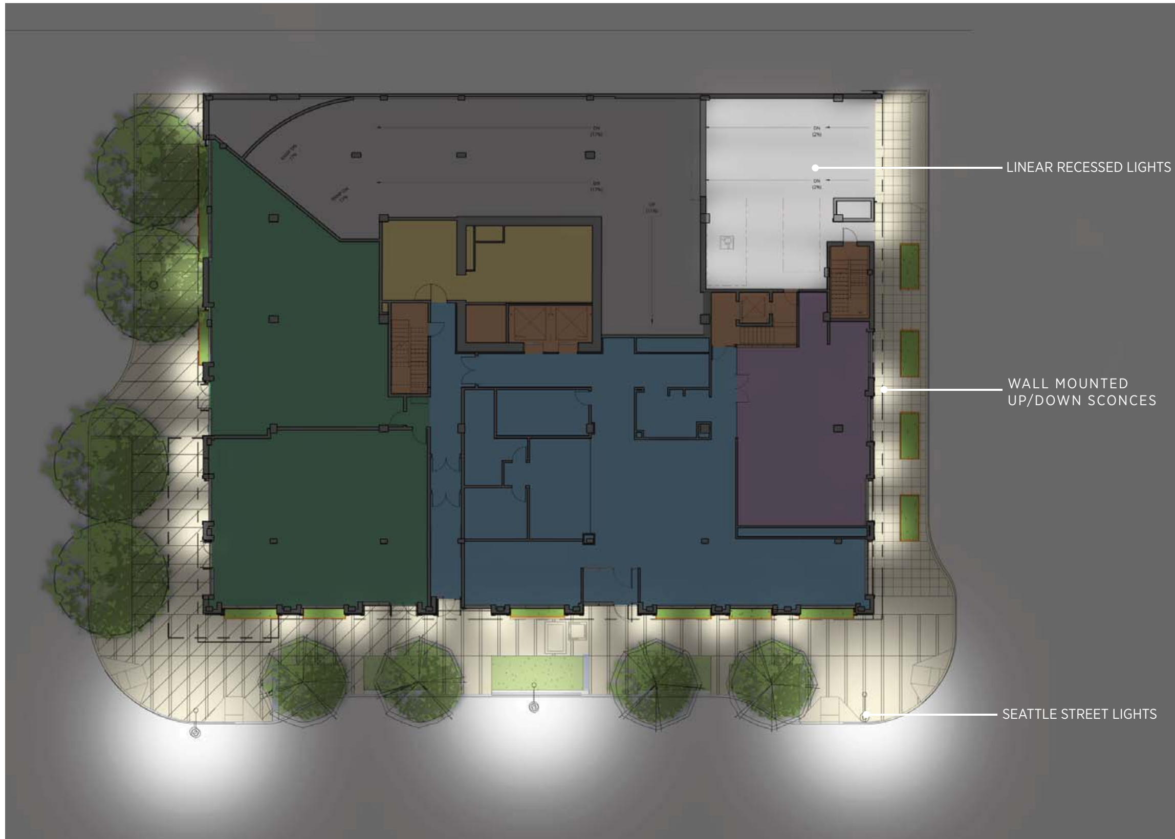
GROUND LEVEL EXTERIOR LIGHTING PLAN
