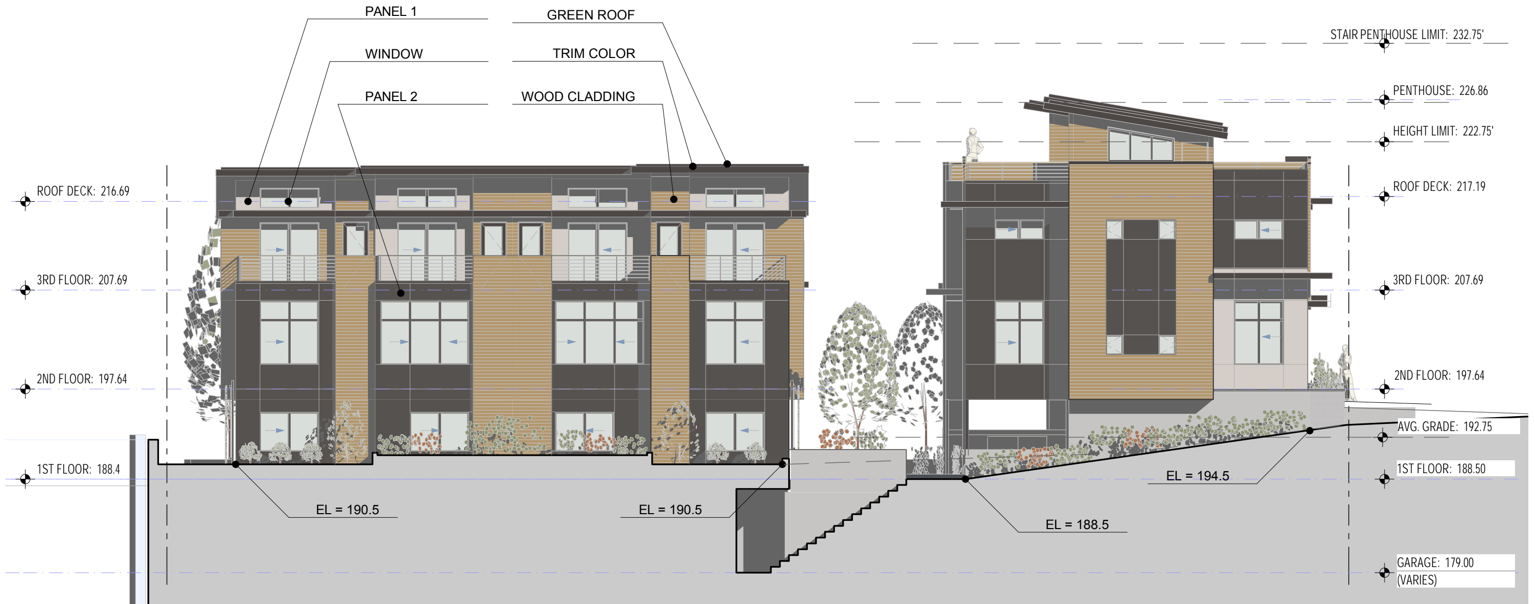
EAST ELEVATION, BUILDINGS 1 & 3
