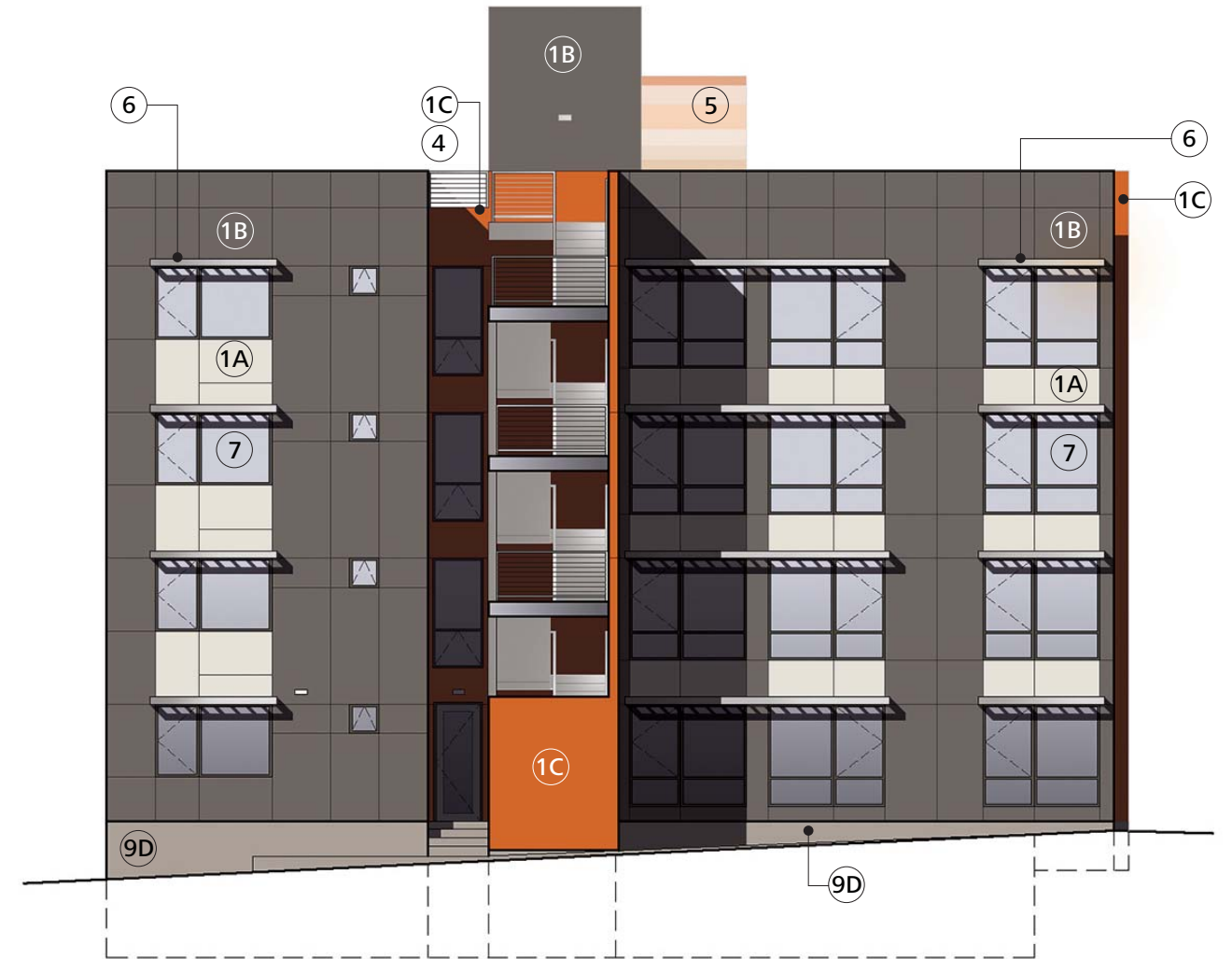
6. SUNSHADES AT SOUTH ELEVATION ONLY WHERE SOLAR EXPOSURE IS MOST SIGNIFICANT
