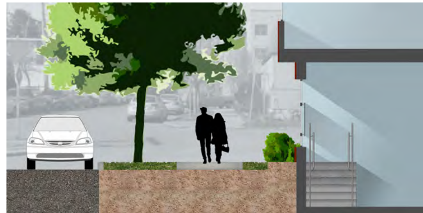
OPTION A SECTION WITH LOWER FLOOR LEVEL FOR RESIDENTIAL SECURITY
