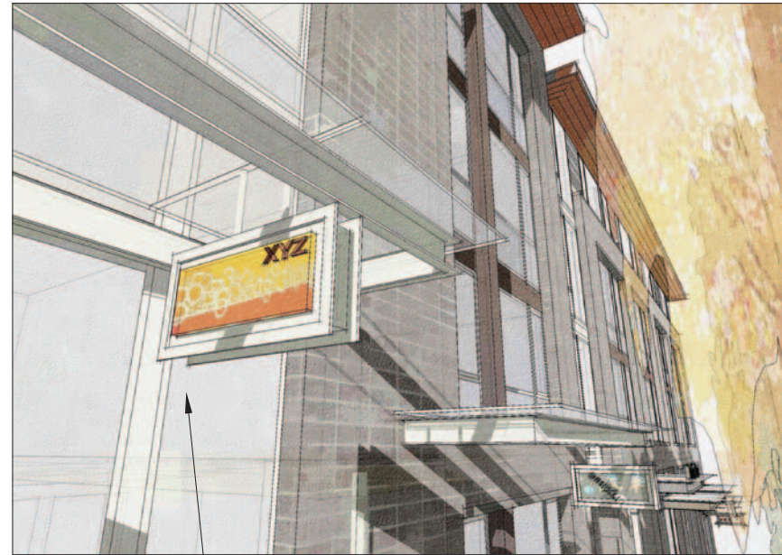
STEEL CHANNEL TO MATCH CANOPY. SUSPEND FROM CANOPY FRAME W/ STEEL RODS (FINISHED TO MATCH CORRUGATED ROOFING MATERIAL)
